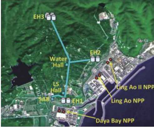
Fig. 1. (color online) Layout of the Daya Bay experiment. Eight antineutrino detectors (ADs) are placed in three experimental halls (EHs). The solid cylinders represent the ADs. There are three nuclear power plants (NPPs): Daya Bay, Ling Ao, and Ling Ao II near EH1 and EH2. Each NPP consists of two reactor cores, shown as the red dots in the figure.
