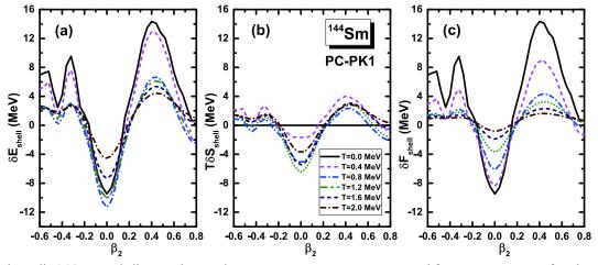
**Fig. 4.** (color online) Neutron shell corrections to the energy  $\delta E_{\text{shell}}$ , entropy  $T\delta S_{\text{shell}}$ , and free energy  $\delta F_{\text{shell}}$  as functions of quadrupole deformation  $\beta_2$  for <sup>144</sup>Sm at different temperatures from 0 to 2 MeV with steps of 0.4 MeV obtained by the constrained CDFT+BCS calculations using PC-PK1 energy density functional.
