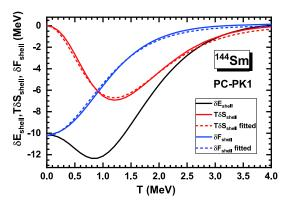
**Fig. 5.** (color online) The temperature dependence of the shell corrections to the energy  $\delta E_{\text{shell}}$  (black line), entropy  $T\delta S_{\text{shell}}$  (red line), and free energy  $\delta F_{\text{shell}}$  (blue line) with corresponding fitted empirical Bohr-Mottelson forms [7] (dashed lines) for the states with minimum free energy in <sup>144</sup>Sm shown in Fig. 3 obtained using the constrained CDFT+BCS calculations applying the PC-PK1 energy density functional.
