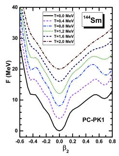
**Fig. 3.** (color online) The relative free energy curves for <sup>144</sup>Sm at different temperatures in the range of 0 to 2 MeV with a step of 0.4 MeV obtained by the constrained CDFT+BCS calculations using the PC-PK1 energy density functional. The ground state free energy at zero temperature is set to zero and is shifted up by 4 MeV for every 0.4 MeV temperature rise.
