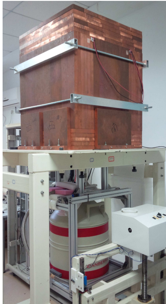
Fig. 1. (color online) HPGe spectrometer with 15 cm copper shielding.
