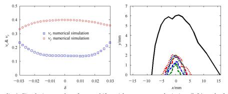
Fig. 7. (color online) Simulation results of tune shifts with momentum deviation (left) and of the momentum dependent DA, for latest version of the PEPX-type lattice for HEPS (mode 2). In the right plot, with  $\delta=0$  (black solid),  $\delta=1\%$  (red dashed),  $\delta=-1\%$  (red dotted),  $\delta=2\%$  (blue dashed),  $\delta=-2\%$  (blue dotted),  $\delta=3\%$  (green dashed) and  $\delta=-3\%$  (green dotted).
