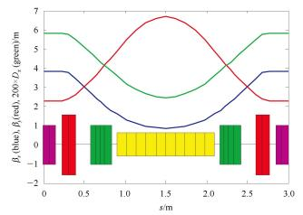
Fig. 3. (color online) Layout and optical function of the 3-m unit cell in middle of the standard 7BA, for the latest version of the PEPX-type lattice for HEPS. Purple blocks represent horizontally focusing sextupoles, red blocks represent horizontally focusing quadrupole, green blocks represent horizontally defocusing sextupoles, and yellow block represents dipole combined with horizontally defocusing gradient.
