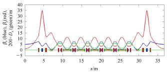
Fig. 1. (color online) Layout and optical functions of a standard 7BA with 7-m ID straight section, for the second version of the PEPX-type lattice for HEPS.
