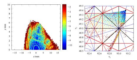
Fig. 8. (color online) The dynamic aperture and frequency map obtained after over 1024 turns for latest version of the PEPX-type lattice for HEPS (mode 2, with sextupole/octupole strengths different from those for Fig. 5). The colors, from blue to red, represent the stabilities of the particle motion, from stable to unstable.
