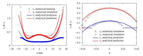
Fig. 6. (color online) Tune shifts with horizontal amplitude (left) and with momentum deviation (right), extracted from the numerical tracking results and the theoretical results, respectively, for latest version of the PEPX-type lattice for HEPS (mode 1).
