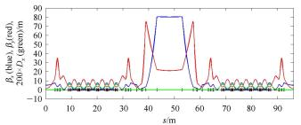
Fig. 2. (color online) Layout and optical functions of two 7BAs with 9.6-m long straight section in between, for the second version of the PEPX-type lattice for HEPS. The optics is matched in such a way that the phase advance of the 9.6-m straight section is different from that of the normal 7-m straight section by  $\Delta \mu_x = 2\pi$  and  $\Delta \mu_y = 0$ .
