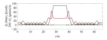
Fig. 4. (color online) Layout and optical functions of two specially designed 7BAs with 10-m long straight section in between, for the latest version of the PEPX-type lattice for HEPS. The phase advance of these two 7BAs is set to  $\mu_x=4\pi$  and  $\mu_y=2\pi$ .
