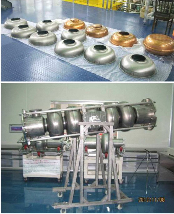
Fig. 5. The formed half-cells and the successfully fabricated 500 MHz 5-cell niobium cavity.
