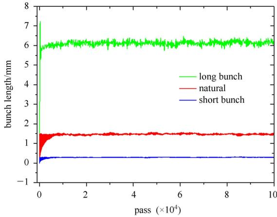
Fig. 4. (color online) ELEGANT tracking results for alternating bunch length scheme in HEPS storage ring. The results for the case without any harmonic cavity are also plotted for comparison.
