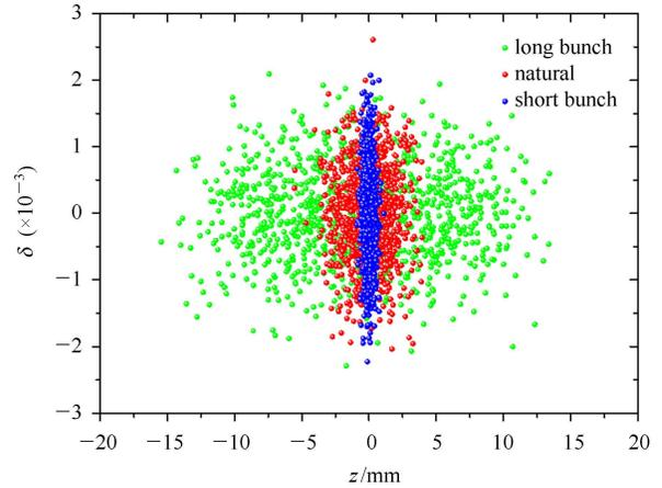
Fig. 5. (color online) ELEGANT tracking results of the particle distributions in longitudinal phase space for alternating bunch length scheme in HEPS storage ring. The results for the case without any harmonic cavity are also plotted for comparison.
