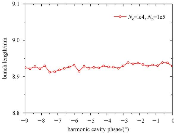
Fig. 2. (color online) Evolution of the bunch length with harmonic cavity phase, obtained with ELEGANT tracking with 10000 micro particles per bunch and over 100 thousand turns.
