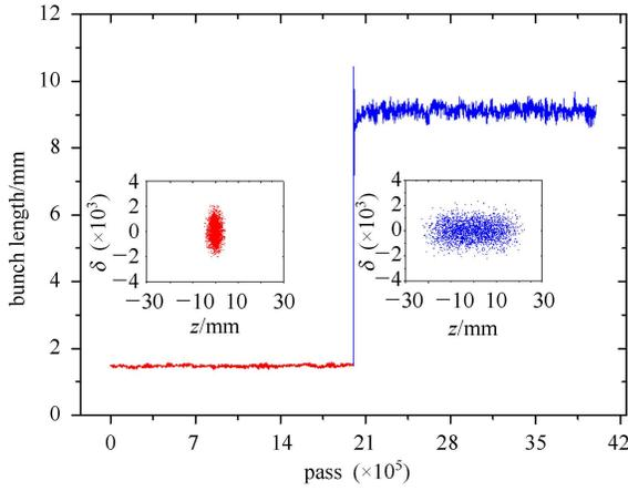
Fig. 1. (color online) ELEGANT simulation results without (red curve) and with (blue curve) harmonic cavity in HEPS storage ring. The final particle distributions in longitudinal phase space are shown in the sub-plots.
