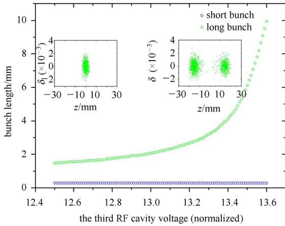
Fig. 3. (color online) Evaluation of the bunch length with normalized voltage of the third harmonic cavity, obtained with ELEGANT.
