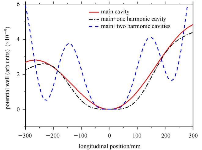
Fig. 6. (color online) RF potential wells for the cases with only the main RF cavity (red curve), with main RF and one harmonic cavity (black curve), and with main RF and two harmonic cavities (blue curve).
