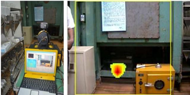
Fig. 10. Searching for radiation source with the precision positioning module.
