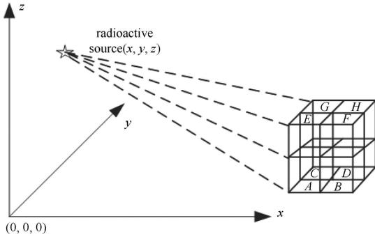
Fig. 5. Positioning in three dimensions with double layer crystal array.
