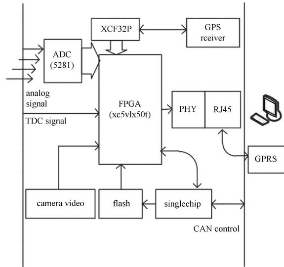
Fig. 2. Hardware structure of data acquisition system.
