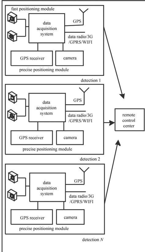
Fig. 1. System structure of the omnidirectional gamma ray system.
