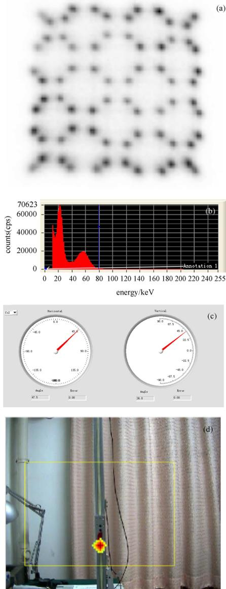
Fig. 9. The experimental results. (a) The flood image, (b) the spectrum, (c) the incident angle of radiation source in horizontal /vertical direction, (d) the fusion image.
