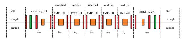
Fig. 2. Schematic of one 7BA supercell.
