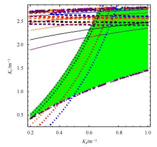
Fig. 4. (color online) Necktie diagram and contour plots of the emittance and the phase advance in  $(K_{\rm f}, K_{\rm d})$  space. The green area represents the region for stable optics. The solid lines, from upper to lower, refer to  $\mu_x = (14/32, 13/32, 12/32, 11/32, 11/32)\pi$ ; the dotted lines, from left to right, refer to  $\mu_y = (3/64, 5/64, 7/64, 9/64, 11/64) \pi$ ; and the dashed lines, from upper to lower, refer to  $\varepsilon_x = (80, 85, 90, 100, 110)$  pm.
