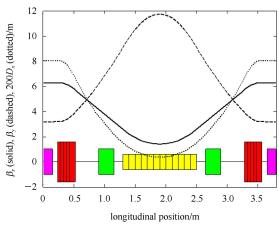
Fig. 5. Optical functions in a modified-TME unit cell with  $(\mu_x, \mu_y) = (13\pi/32, 7\pi/64)$ .
