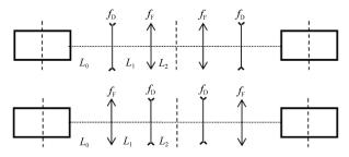
Fig. 1. Two TME-like cell configurations, with QD closer to the dipole in a modified-TME cell (the upper plot), and with QF closer to the dipole in a conventional TME-like cell or in a TME cell (the lower plot).
