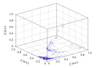
Fig. 8. Pareto-optimal solutions obtained after 500 generations with NSGA-II. Three objectives are used, with  $f_1$ ,  $f_2$ , and  $f_3$  characterizing the detune, chromaticity and resonance terms, respectively. The star denotes the best solution found, which provides large dynamic aperture.
