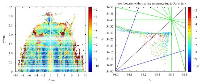
Fig. 9. (color online) The dynamic aperture and frequency map obtained after tracking of 1024 turns with AT code for BAPS ring lattice by using 12 families of sextupoles and 6 families of octupoles with strengths obtained by NSGA-II. The colors from blue to red, represent the stabilities of the particle motion, from stable to unstable.
