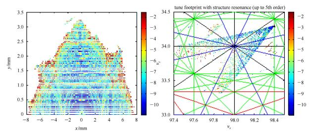
Fig. 7. (color online) The dynamic aperture and frequency map obtained after tracking of 1024 turns with AT code for BAPS ring lattice with only two families of chromaticity-correction sextupoles. The colors from blue to red, represent the stabilities of the particle motion, from stable to unstable.
