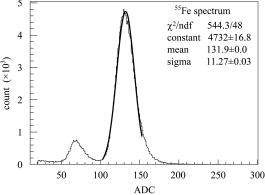
Fig. 3. A typical  $^{55}$ Fe energy spectrum, in Ar/isobutane(95/5) mixture. The energy resolution is  $2.35 \times 11.27/131.9 = 20.08\%$ .
