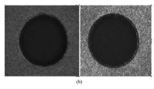
Fig. 1. Images of the THGEM plates. (a) The standard THGEM structure; (b) A single hole before (left) and after (right) the processes described in the text. The treated rim is less than 10 μm.
