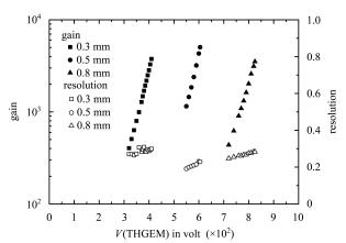
Fig. 2. The gain and energy resolution of single THGEM. In an Ar/isobutane(95/5) mixture, the drift field is 1 kV/cm and induction field 2.7 kV/cm.
