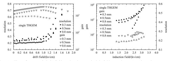
Fig. 4. The influences of drift (left) and induction (right) fields on the gain and resolution in an Ar/isobutane(95/5) mixture. The THGEM thickness is 0.5 mm and the voltage is 595 V.
