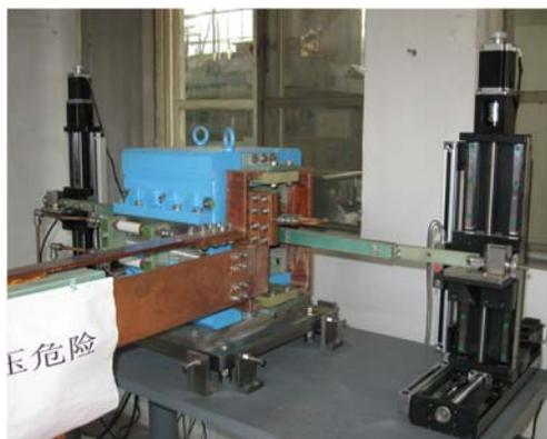
Fig. 11. The experiment of search coil measuring magnetic field.
