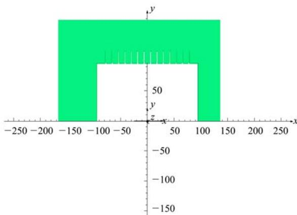
Fig. 12. The optimized structure of the end plate.
