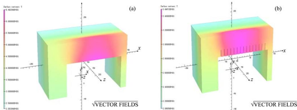
Fig. 7. The distribution of the temperature in the end plates. (a) The end plate without slit cut; (b) The end plate with 15 slit cuts.
