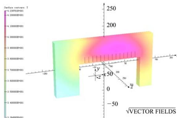
Fig. 13. The distribution of the temperature in the end plate.
