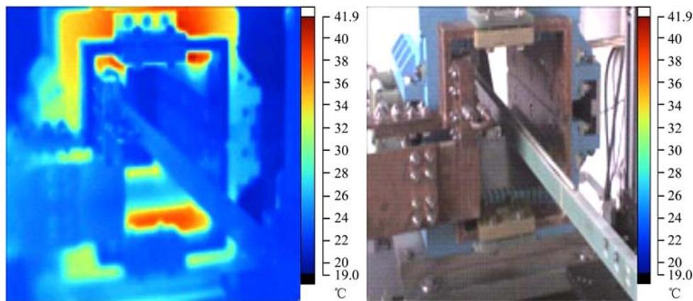
Fig. 10. The measurement of temperature in the end plates.
