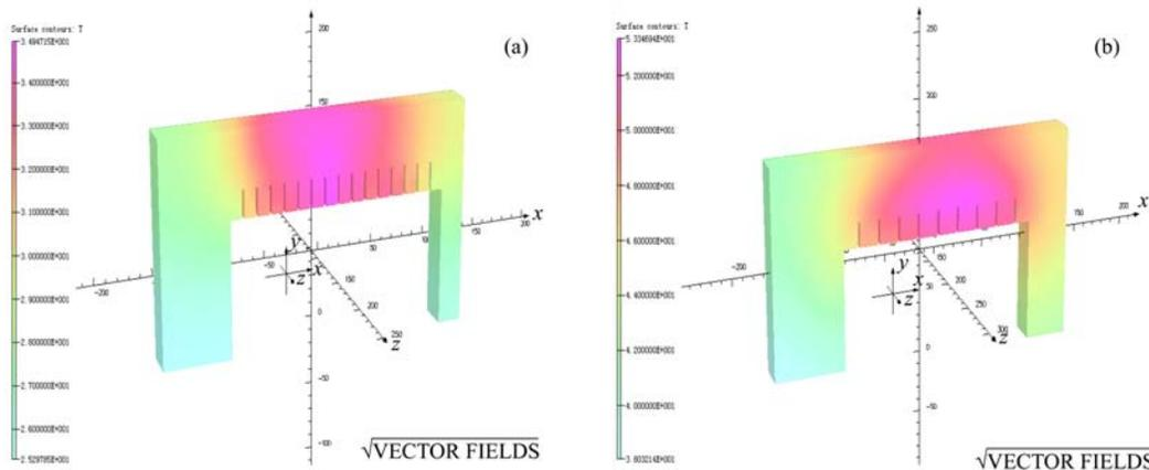
Fig. 8. The distribution of the temperature in the end plates. (a) The end plate with thin slit cuts; (b) The end plate with wide slit cuts.
