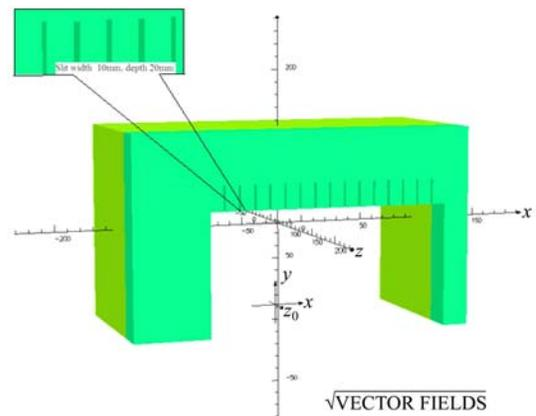
Fig. 5. The 1/4 BH magnet finite element model.
