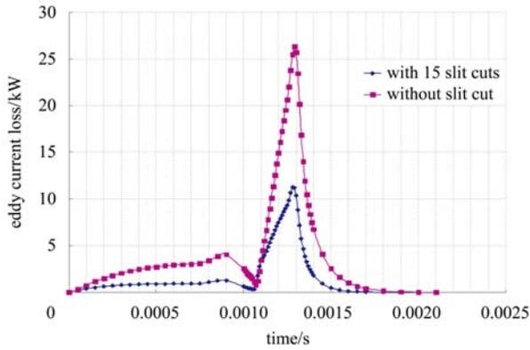
Fig. 6. The calculated results of the eddy current losses.
