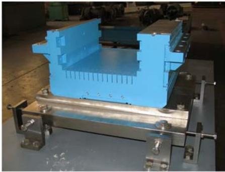
Fig. 3. The slit cuts in the end plates of the lower half core.
