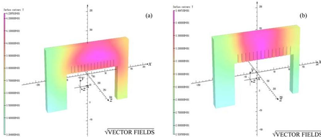
Fig. 9. The distribution of the temperature in the end plates. (a) The end plate with 14 slit cuts; (b) The end plate with 15 slit cuts.
