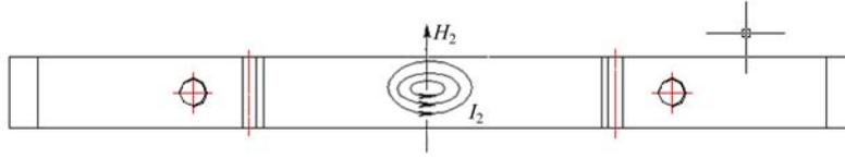
Fig. 4. The path of eddy current in the planform of the end plate.
