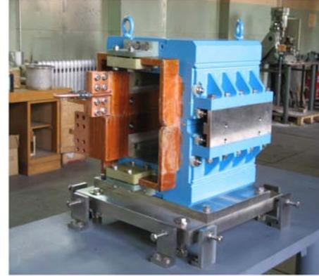
Fig. 2. The assembly of the prototype BH magnet.
