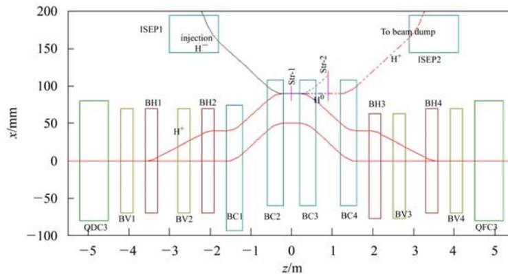
Fig. 1. The component layout of the injection.
