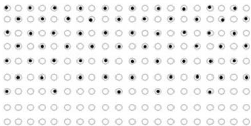
Fig. 4. Ions in the Si lattice after two-step annealing and no point discharge occurs. Blank circles represent silicon atoms and circles with a dark point inside represent implanted ions.
