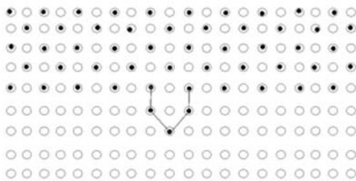
Fig. 3. Ions in the Si lattice after a one-step anneal, and the ion-channel effect occurs. Blank circles represent silicon atoms, and circles with a dark point inside represent implanted ions.
