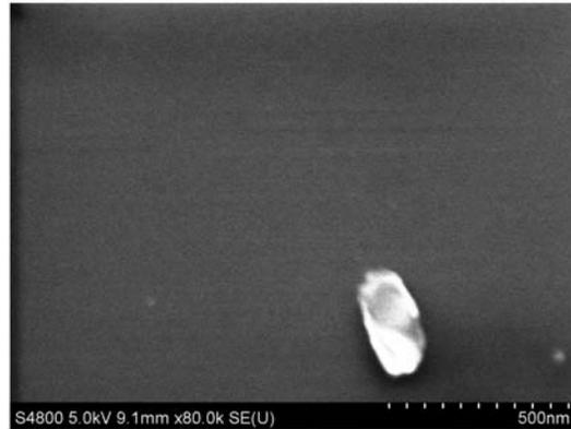
Fig. 5. A scanning electron micrograph of this interface shows few defects after two-step RTA.
