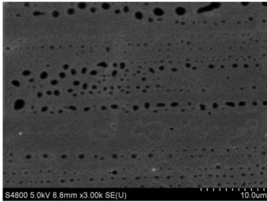
Fig. 2. A scanning electron micrograph of this interface shows a lot of defects after only one-step RTA.
