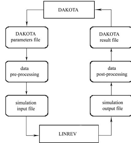
Fig. 2. The loosely coupled interface between DAKOTA and the simulation code LINREV.
