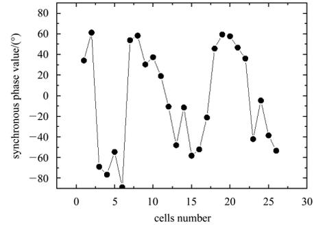
Fig. 4. The array of synchronous phase in the APF DTL.
