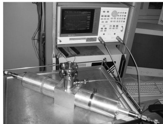
Fig. 4. A photograph of the coaxial transmission line with the HOM coupler.
