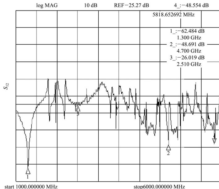
Fig. 7. The stop band characteristics of the TTF type HOM coupler.
