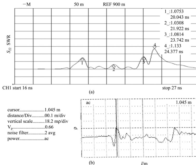
Fig. 5. Reflection coefficient of coaxial transmission line measured by 1502C metallic TDR.
