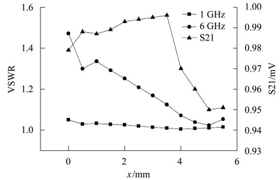
Fig. 2. VSWR and scatter parameter as a function of  $x$  at 1 GHz and 6 GHz while the diameter of the outer conductor change from 18.4 mm to 23 mm.
