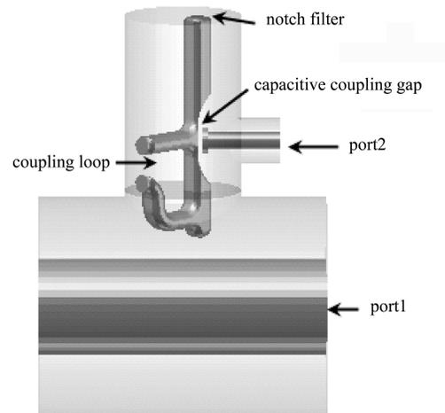
Fig. 1. Model of the HOM coupler and the coaxial transmission line for simulation.
