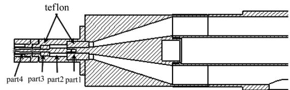
Fig. 3. Structure of the coaxial transmission line with the step part.
