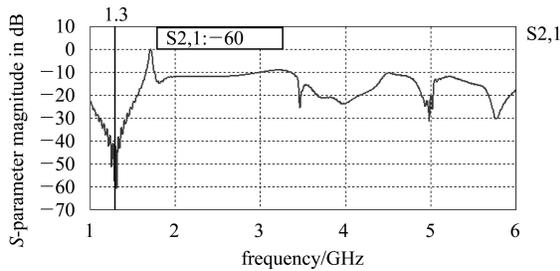
Fig. 6. The scattering parameter of the HOM coupler with the coaxial transmission line.
