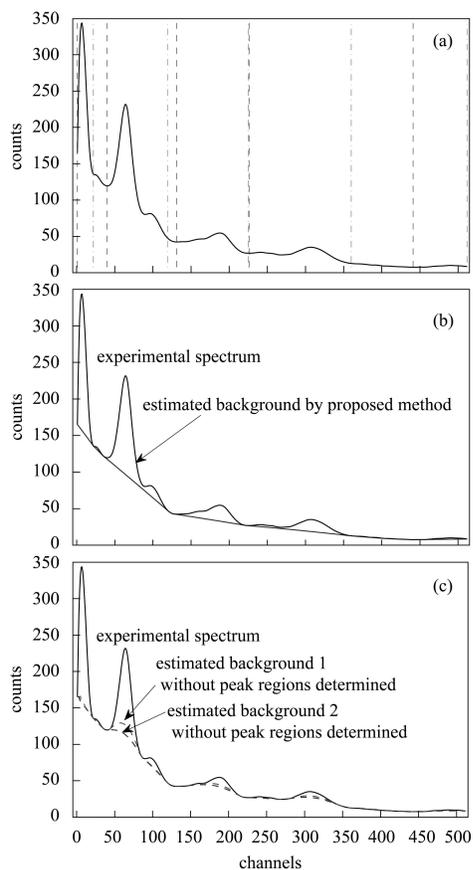
Fig. 6. Estimation of the peak regions in the experimental spectra detected by the NaI detector. (a) Estimation of the peak regions in the experimental spectra with the proposed method. Dashed line: Start point of the current region; dashed dot line: End point of the current region; (b) Background estimation using the SNIP method in each calculated region. (c) Background estimation using SNIP without the peak regions determined.
