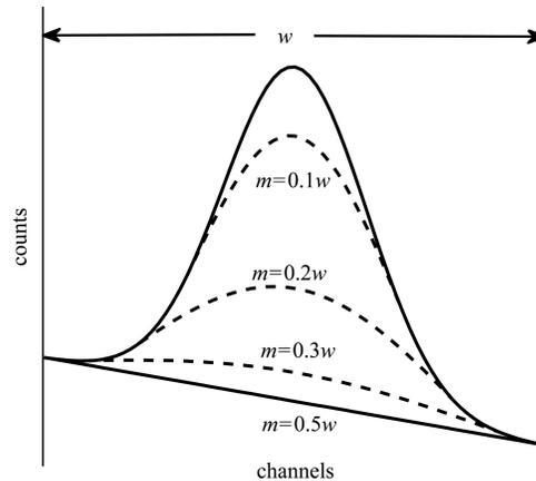
Fig. 1. Background elimination with different  $m$  using the SNIP method. Here,  $w$  is the real width of the object.
