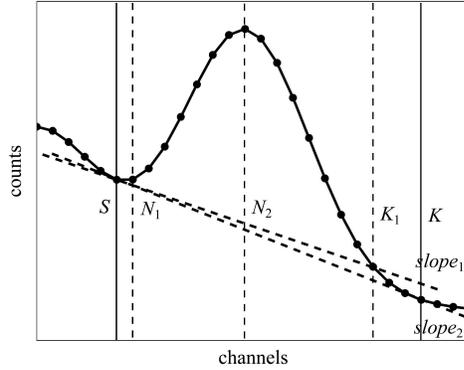
Fig. 4. The first correction of the heuristic approach to get the real end point of a current region.
