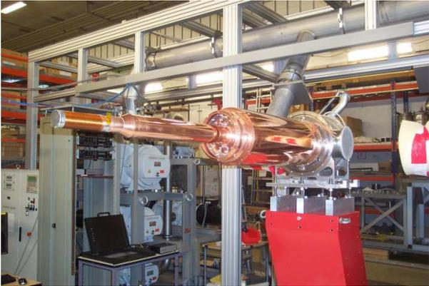
Fig. 8. The new dilution refrigerator for the Crystal Ball Frozen Spin Target.
