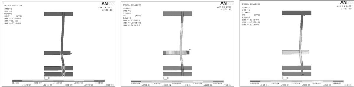
Fig. 6. Stress distribution, horizontal and vertical displacements of the support post after being cooled down (Unit: stress—Pa, deformation—m).
