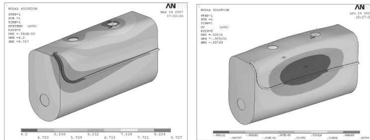
Fig. 3. Temperature distribution and deformation along the horizontal & axial direction of the 5 K shield with a helium flow of 0.08 g/s (Unit: temperature—K, deformation—m).
