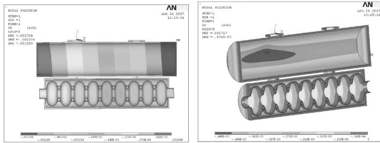
Fig. 5. Horizontal deformation of the 2 K system after being cooled down (Unit: m).
