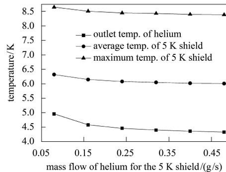
Fig. 4. Variation of outlet temperature of the cooling helium, average and maximum temperature of the 5 K shield with the different mass flow of the cooling gas.
