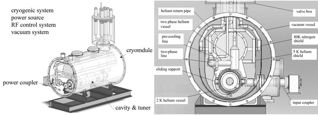
Fig. 1. Structure of the China test cryomodule for ILC.
