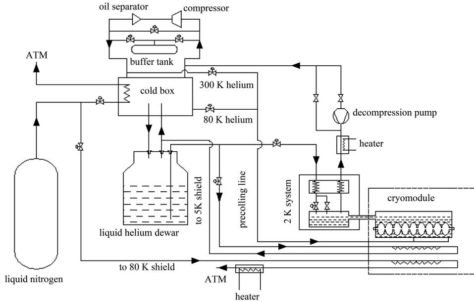
Fig. 2. Cryogenic flow diagram of the test cryomodule.
