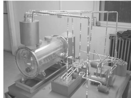
Fig. 7. A scaled model for the China test cryomodule system.
