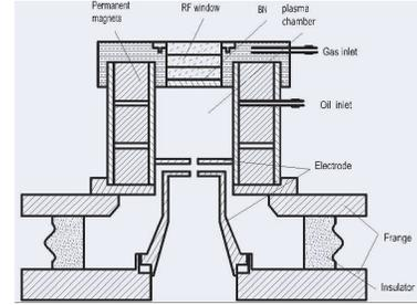
Fig. 2. A schematic plot of the ECR ion source.
