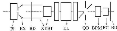
Fig. 4. The new system for ISR RFQ-1000 upgrading. (IS: ion source; EX: Extraction; BD: Beam diaphragm; XYST: X and Y steer; EL: Einzel lens; QD: Quadruple diaphragm; BPM: Beam position monitor; FC: Faraday cup).
