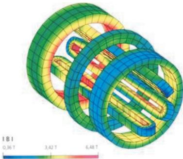
Fig. 1. Magnetic flux density on the sextupole and solenoids of SERSE under design currents.
