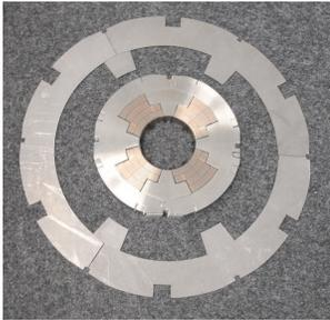
Fig. 4. Collar for the MS-ECRIS sextupole and collared CERN LHC MQY sample for size comparison.
