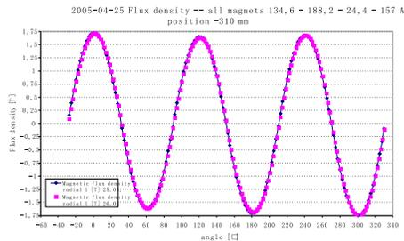
Fig. 6. Radial magnetic field of SECRAL measured with Hall probes.
