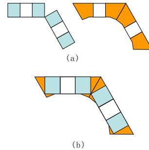
Fig. 2.  $1/3$  (two coils building  $120^\circ$ ) of the cross section of a sextupole; (a) comparison of racetrack and 'advanced' racetrack; in the 'advanced' racetrack geometry the conductor is placed more effectively; (b) direct comparison of the conductor placements.
