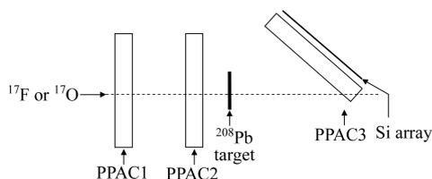
Fig. 1. The schematic figure of experimental setup.
