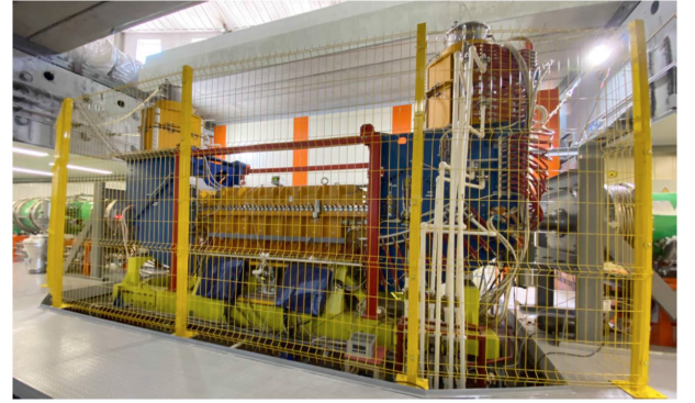
Fig. 2. (color online) Image of the Booster electron cooling system with the 2.5 m cooling section designed for a maximum electron energy of 50 keV.
