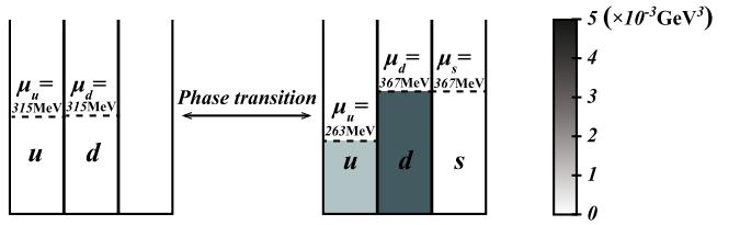
**Fig. 5.** (color online) Schematic illustration of the change of chemical potentials and quark number densities in the chiral phase transition. Quark number densities are represented by darkness.
