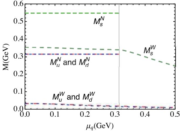
**Fig. 3.** (color online) Effective masses of quarks for both Nambu and Wigner solutions. The superscript 'N' means Nambu solution, 'W' means Wigner solution.
