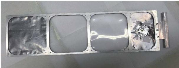
**Fig. 1.** (color online) Samples and sample holder. From left to right: carbon sample, empty target, CH<sub>2</sub> sample, and  $\alpha$  sources.
