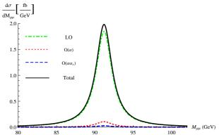
Fig. 5. (color online)  $\mu^+\mu^-$  invariant mass spectrum at  $\sqrt{s}$ =240 GeV, at various levels of perturbative accuracy.
