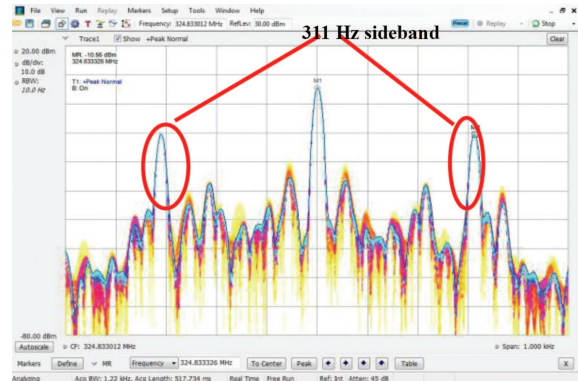
Fig. 3. (color online) Spectrogram of the pick-up signal of the Spoke012 cavity on working, which shows that the 311 Hz sideband has been driven.
