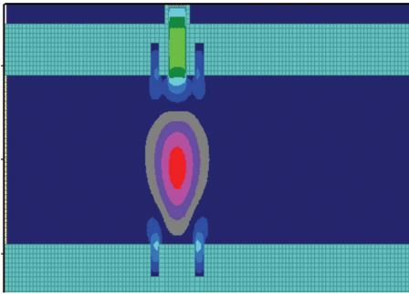
Fig. 1. (color online) Overmoded input cavity structure and its electric field distribution.
