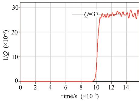
Fig. 5. (color online)  $1/Q$  curve of the overmoded input cavity.
