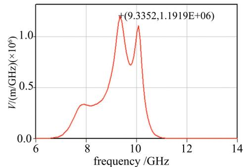
Fig. 4. (color online) Resonant characteristic of the overmoded input cavity.
