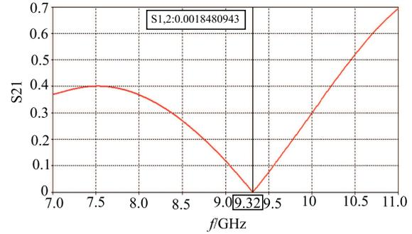
Fig. 2. (color online)  $S_{21}$  curve of the resonant reflector.
