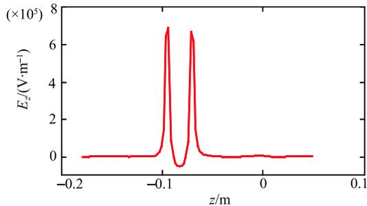
Fig. 7. (color online) Electric field distribution along the beam path.
