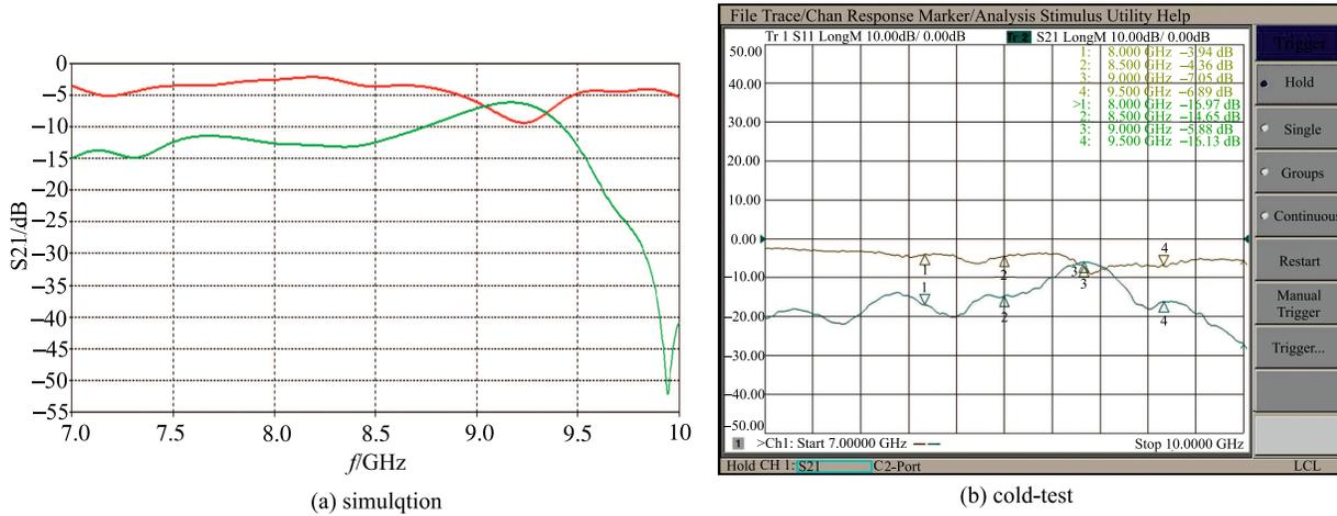
Fig. 10. (color online) S11 and S21 curves of the overmoded input cavity.
