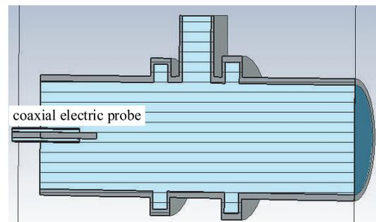
Fig. 9. (color online) Simulation model of the overmoded input cavity for cold test.
