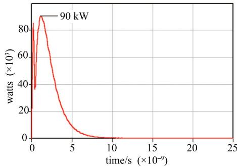
Fig. 6. (color online) RF power injected into the input cavity without electron beam.
