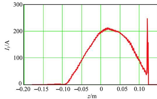
Fig. 8. (color online) The fundamental harmonic current distribution modulated by input cavity.
