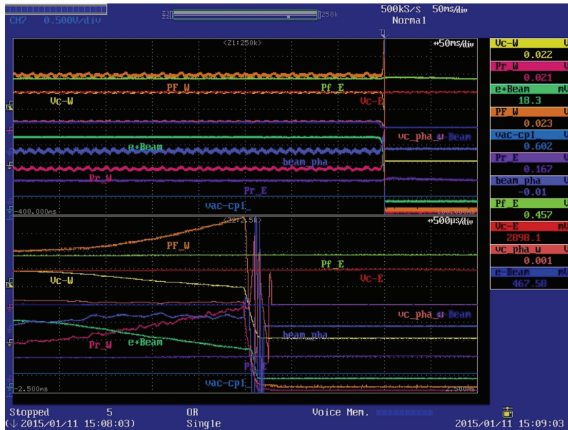
Fig. 8. (color online) Beam trip image recorded by the multi-channel oscilloscope (201501111508). (Vc-W: BPR cavity voltage; Pr-W: BPR cavity reflection RF power; e^+ Beam: positron intensity; PF-W: BPR cavity forward RF power; vac-cpl: BPR cavity power coupler vacuum pressure; Pr_E: BER cavity reflection RF power; beam.pha: positron phase; Pf_E: BER cavity forward RF power; Vc-E: BER cavity voltage; vc pha_w: BPR cavity phase; e-beam: electron intensity).
