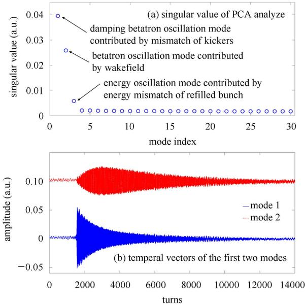
Fig. 5. (color online) (a) Singular value of PCA analysis for position signal; (b) Temporal vectors of the first two modes.
