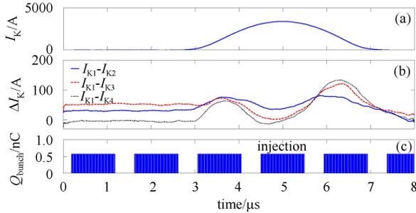
Fig. 2. (color online) Timing relation between bunch train and excitation current waveform.
