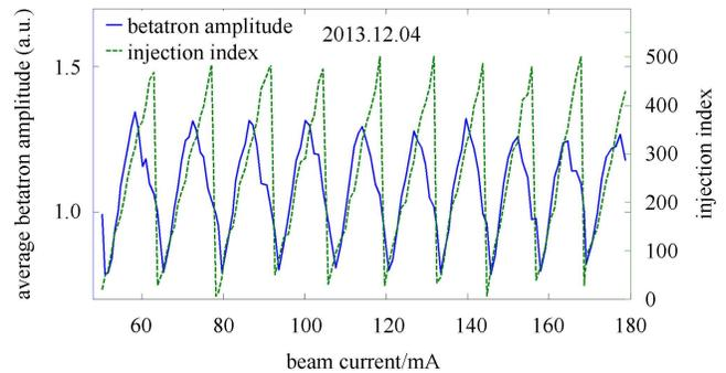
Fig. 11. (color online) Relationship between betatron oscillation amplitude, injection bunch index, and average current.
