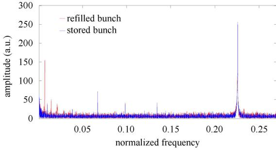
Fig. 4. (color online) Spectrum of the refilling bunch and the stored bunch position signals.
