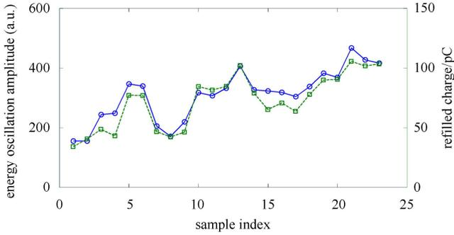
Fig. 8. (color online) Relationship between oscillation amplitude and refilled charge.
