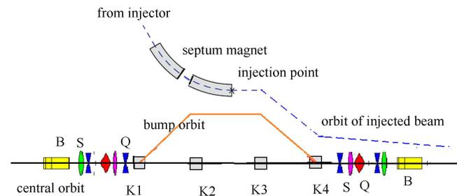
Fig. 1. (color online) Layout of the SSRF injection system.
