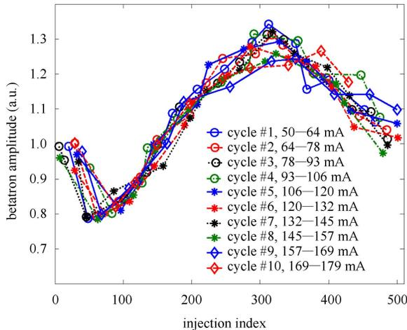
Fig. 12. (color online) Relationship between the amplitude of average residual oscillation and the index of the injected bunch over 10 cycles.
