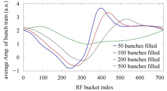
Fig. 10. (color online) Relationship between the average residual amplitude and the index of the injected bunch.
