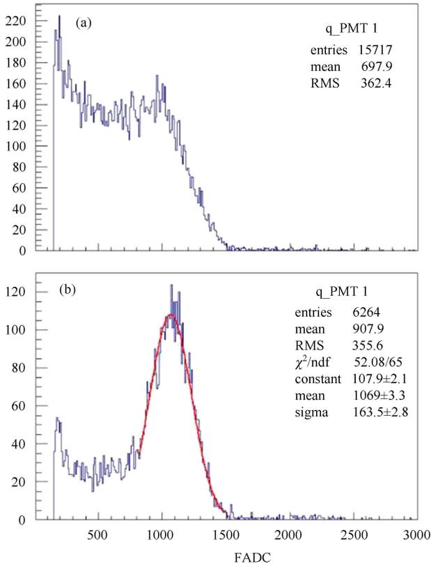
Fig. 3. LS energy spectrum of non-coincidence detection (a) and coincidence detection (b).
