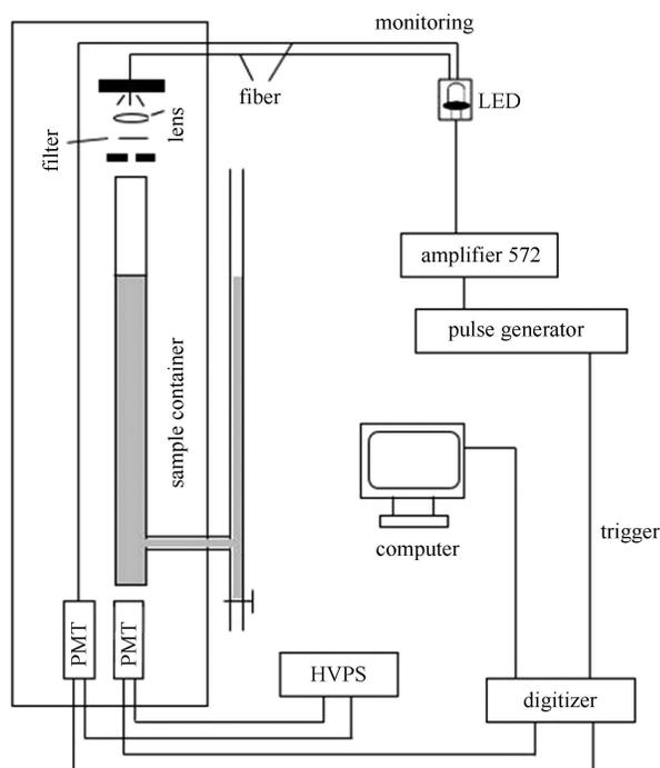
Fig. 6. Attenuation length measurement device.
