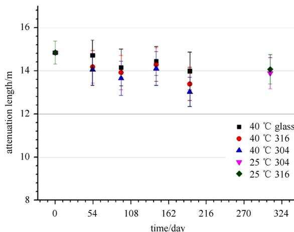
Fig. 7. Attenuation length of aging LS.
