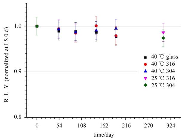
Fig. 5. The result of relative light yield (R. L. Y) measurement.
