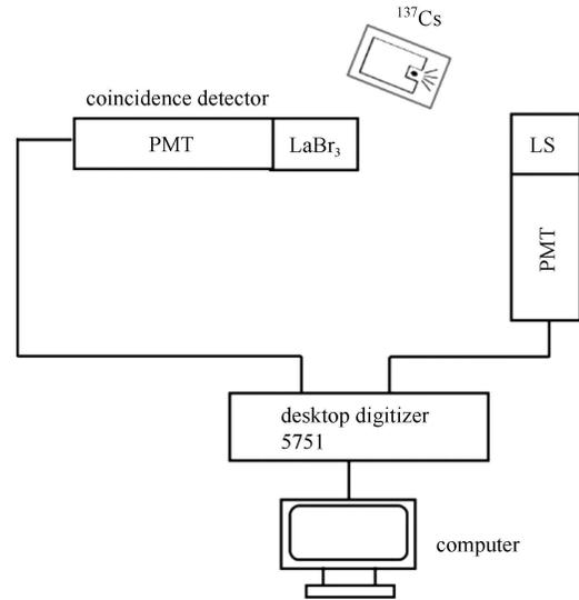
Fig. 4. Experimental setup for measuring the LS light yield.
