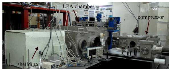
Fig. 5. Laser plasma experimental station.
