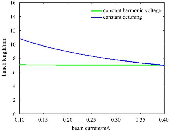
Fig. 11. Reduced bunch length vs. beam current for the constant detuning ( $87.5^\circ$ ) and the constant voltage (218 kV) scenarios.
