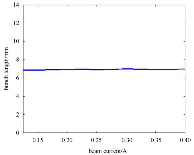
Fig. 8. Minimum bunch length at each beam current.
