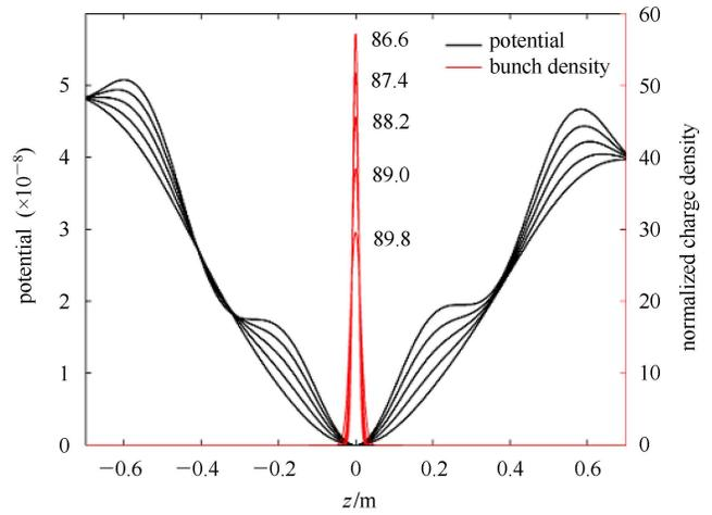
Fig. 4. Potential and density distributions for several values of the tuning angle.
