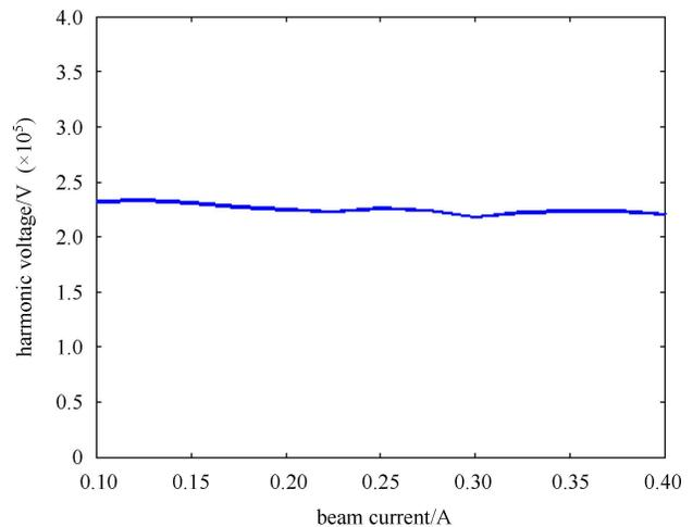
Fig. 9. Optimum harmonic voltage at each beam current.
