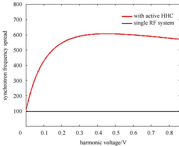
Fig. 13. Frequency spread variation with the voltage of the active HHC.
