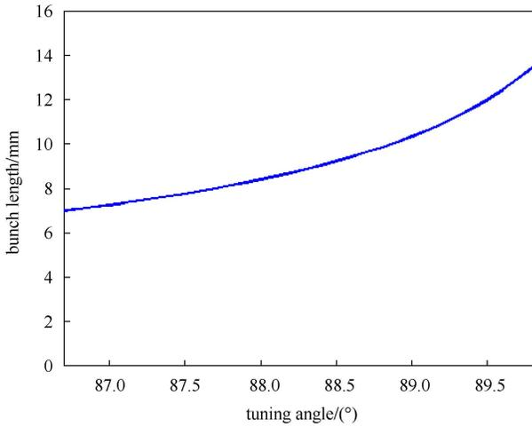
Fig. 6. Bunch lengths for several tuning angles greater than  $86.7^\circ$ .
