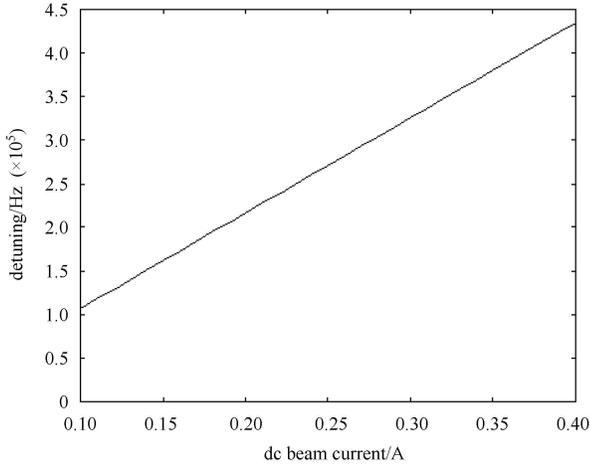
Fig. 10. Relationship of detuning to beam current for the constant voltage scenario.
