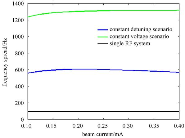
Fig. 12. Frequency spread for the constant detuning and the constant voltage scenarios.
