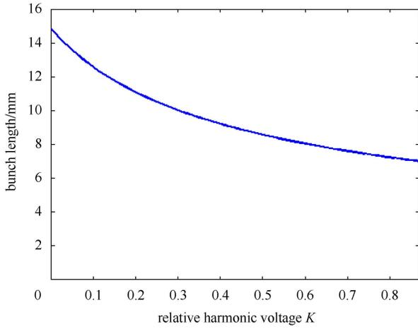
Fig. 3. Bunch lengths for several values of  $K$  smaller than the optimum value of 0.86.
