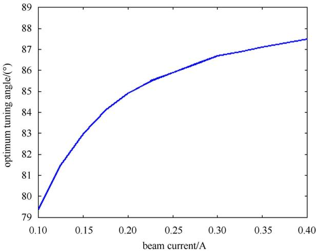
Fig. 7. Optimum tuning angle for each beam current.
