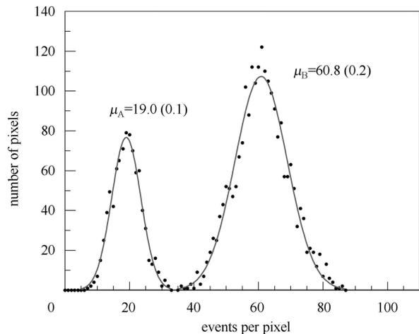
Fig. 3. The modified greyscale spectrum. This spectrum shows the event density distribution after removing the grinding head.  $\mu_A$  and  $\mu_B$  are the fitted average events per pixel in the blocked and unblocked parts respectively. The values in the brackets are the RMS deviations.
