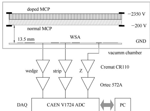
Fig. 1. The imaging detector and electronics system.
