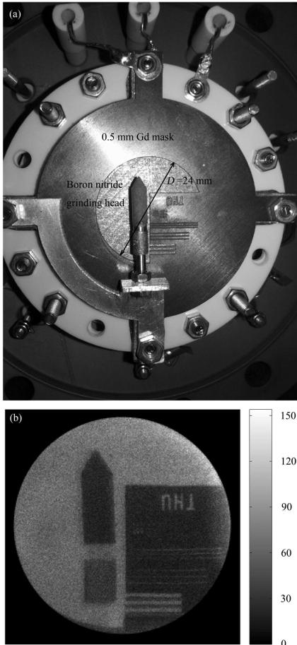
Fig. 2. Imaging objects and results. The imaging objects are fixed in the vacuum chamber. As the neutron flux is very low, in order to get imaging of desirable quality within acceptable acquisition time we selected objects of high contrast for thermal neutrons: the boron nitride grinding head and 0.5 mm Gd mask shown in (a). In (b), the pixel size is 100  $\mu\text{m}$ .
