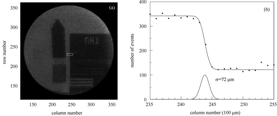
Fig. 4. The derived spatial resolution. In (a), the length of each grid is 3 pixels. The edge within the white box was fitted using error function. The number of events in (b) is the sum of 6 adjacent rows within one column. This was done to suppress the statistical fluctuation at the expense of spatial resolution loss. The RMS of the derivative (Gaussian function) is  $72 \mu\text{m}$ .
