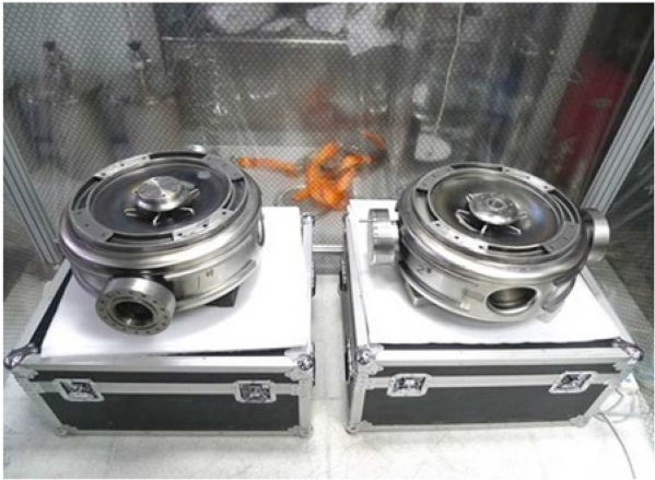
Fig. 7. Two bare Spoke012 prototype cavities fabricated in November 2012.
