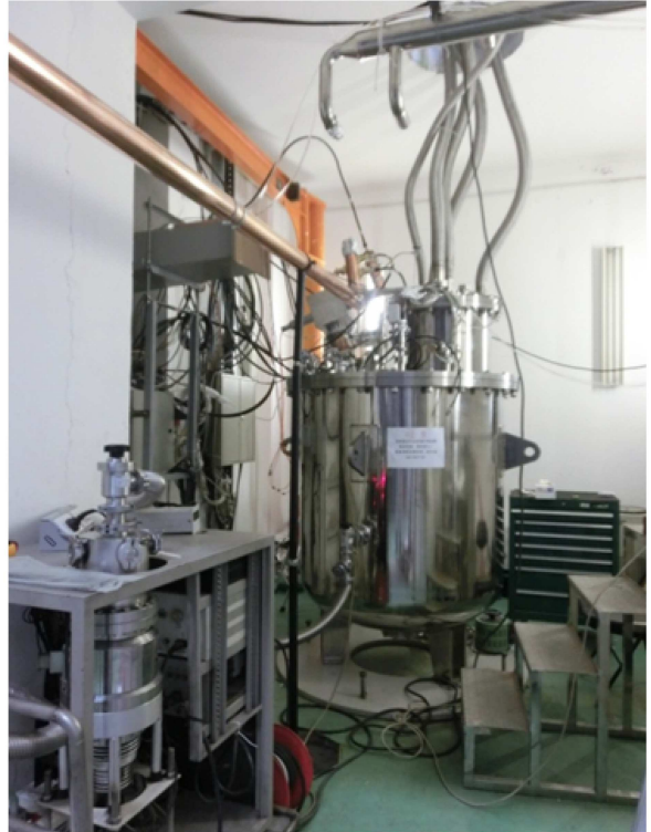
Fig. 9. The cryomodule of Spoke012 with cavity.
