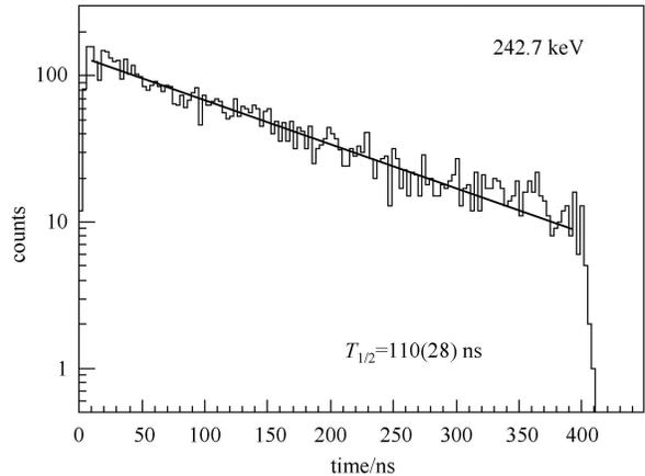
Fig. 2. Least square fitting to the decay curve of the 242.7 keV transition.
