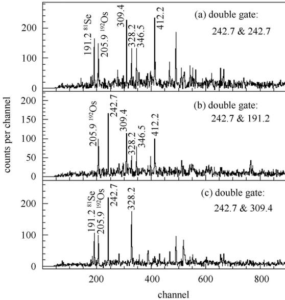
Fig. 4.  $\gamma$ -ray coincidence spectra produced using double gates on the (a) 242.7 and 242.7 keV lines, (b) 242.7 and 191.2 keV lines, (c) 242.7 and 309.4 keV lines. The 205.9 and 191.2 keV transitions are from the target nucleus  $^{192}\text{Os}$  (random coincidence) and the partner nucleus  $^{81}\text{Se}$  (see text), respectively.
