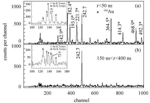
Fig. 1. Spectra gated on the 242.7 keV transition showing  $\gamma$ -rays in prompt [panel (a)] and delayed [panel (b)] coincidence with the 242.7 keV transition. Contaminations from  $^{194}\text{Au}$  are marked with asterisks.
