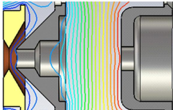
Fig. 5. (color online) The equipotential lines of CYCLONE30 extraction system.
