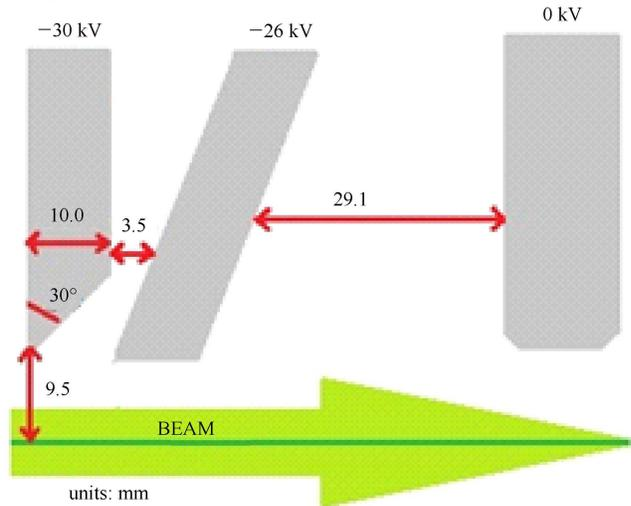
Fig. 4. (color online) Some parameters of the triode extraction system for the present accelerator structure and dimensions.
