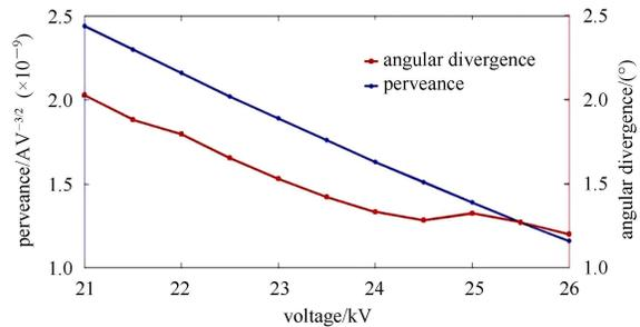
Fig. 8. (color online) Influence of the second electrode voltage on the beam perveance and rms angular divergence.
