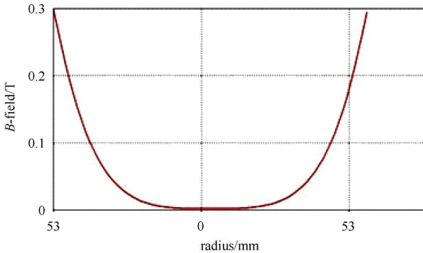
Fig. 3. (color online) Magnetic field density profile along the radius through the pole tips for  $N=10$ .
