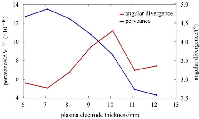
Fig. 6. (color online) Influence of the plasma electrode thickness on the beam perveance and rms angular divergence.
