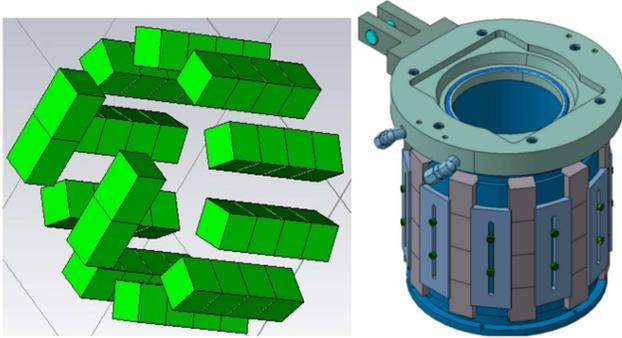
Fig. 1. Distribution of the magnets and the structure of the discharge chamber.
