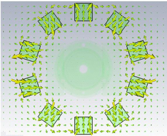
Fig. 2. (color online) The magnetic field distribution in the discharge chamber.
