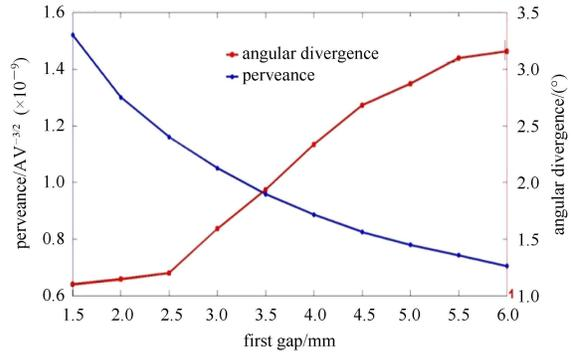
Fig. 7. (color online) Influence of the first gap width on the beam perveance and rms angular divergence.
