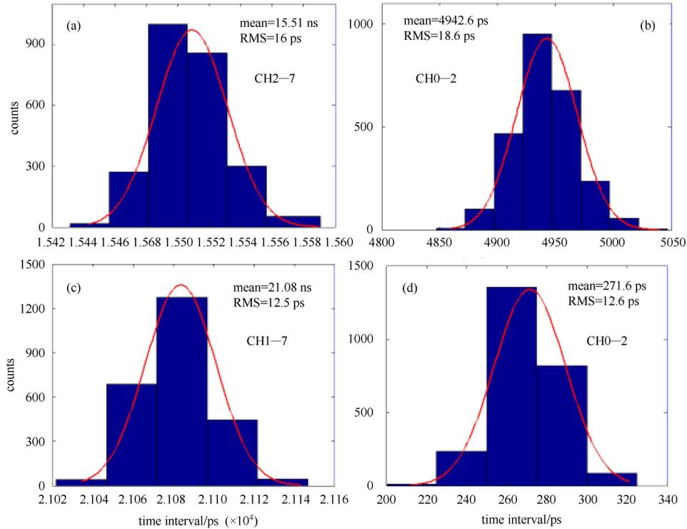
Fig. 6. Time measuring resolution for different HPTDCs (without FEE). (a) HPTDC0; (b) HPTDC1; (c) HPTDC5; (d) HPTDC8.
