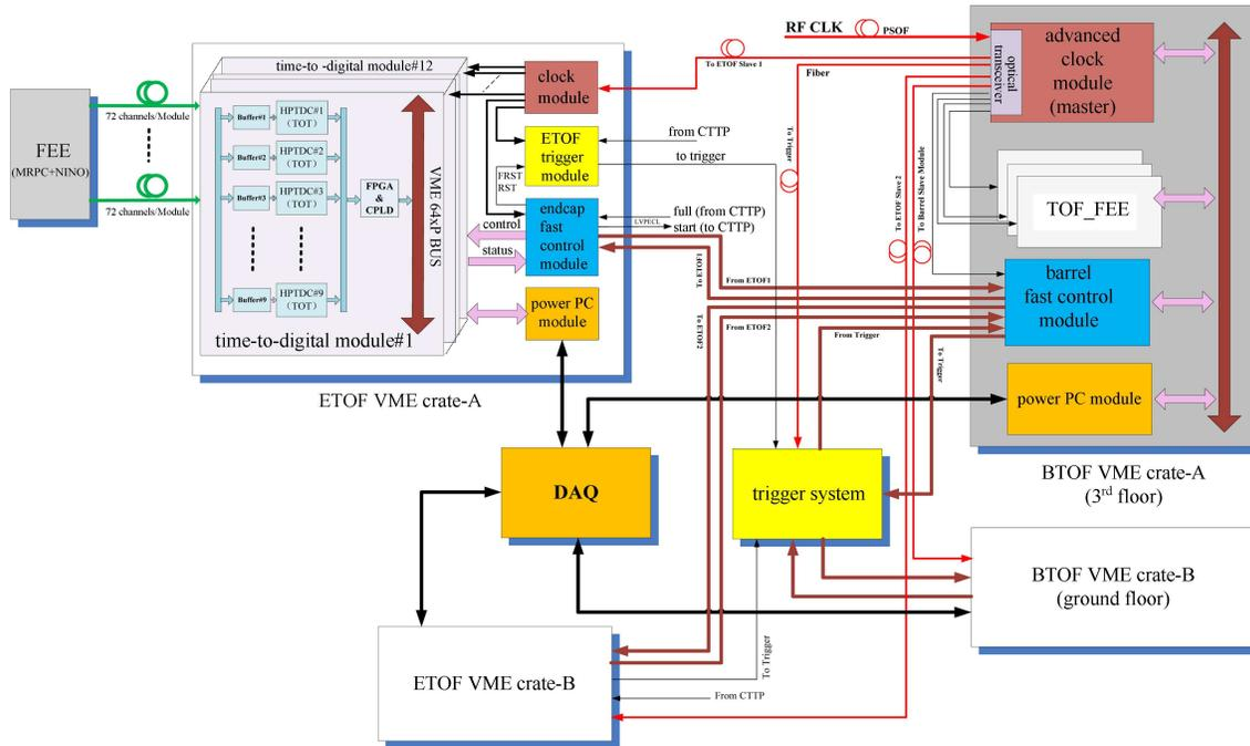
Fig. 1. The architecture of the time digitizing system for the ETOF upgrade.
