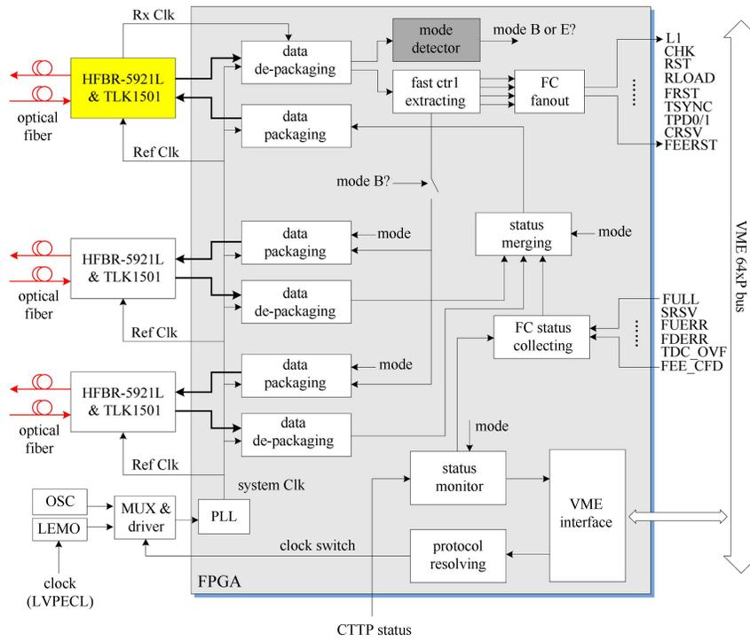
Fig. 3. Structure of fast control module.
