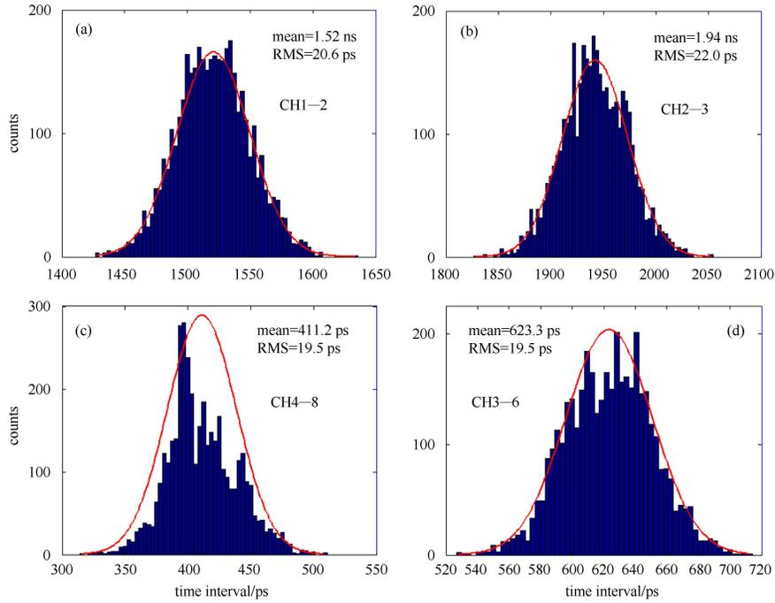
Fig. 7. Time measuring resolution for different HPTDCs (with FEEs). (a) HPTDC2; (b) HPTDC3; (c) HPTDC4; (d) HPTDC8.
