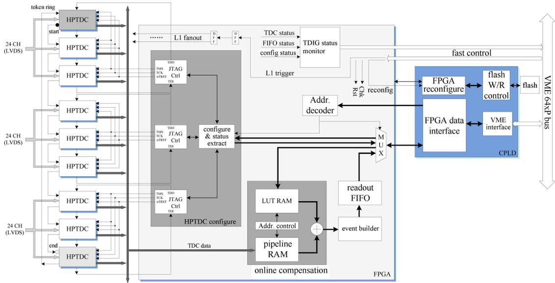
Fig. 2. Structure of TDIG module.
