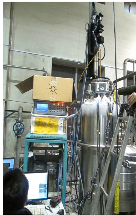
Fig. 8. Ongoing vertical test for the superconducting magnet.
