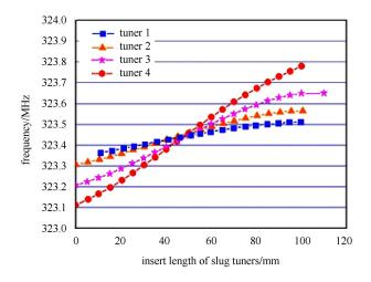
Fig. 3. The frequency shift caused by slug tuners.
