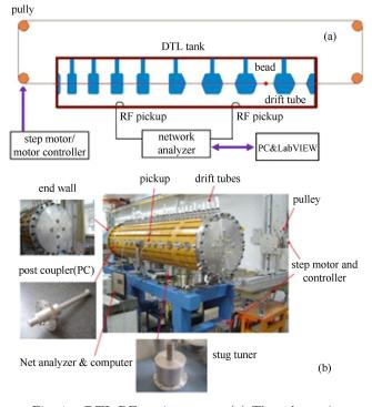
Fig. 1. DTL RF tuning setup. (a) The schematic diagram of a field-measurment; (b) the apparatus photo of DTL RF tuning.
