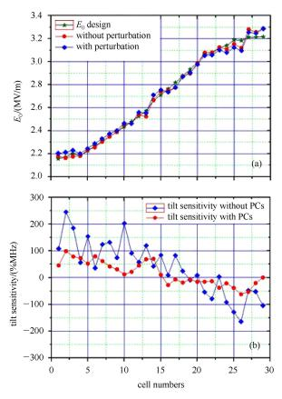
Fig. 8. CSNS DTL1RF tuning results for cold measurement. (a) Field flatness; (b) tilt sensitivity.
