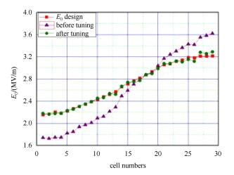
Fig. 4. The field profiles before and after tuning.
