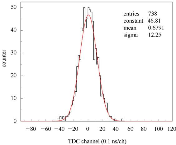
Fig. 5. The time resolution of the LPMWPC.
