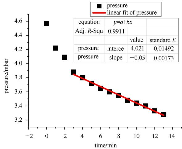
Fig. 2. Gas leakage rate of the LPMWPC is about 0.05 mbar/min when the pressure ranges from 3.88 mbar to 3.28 mbar.
