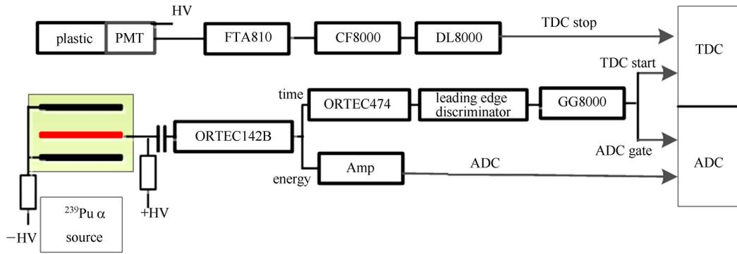
Fig. 3. The time resolution measurement system.
