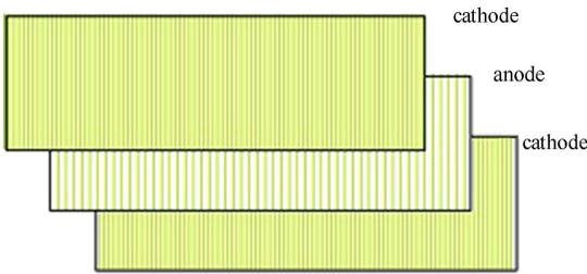
Fig. 1. Structure of the LPMWPC.
