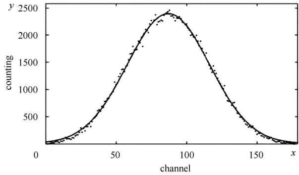
Fig. 7. Gaussian statistical distribution obtained by the M sequence method (the fitting function  $y=2394\exp(-((x-87)/41)^2)$ ,  $\chi^2/(N-1) = \sum_{i=1}^n \frac{(y_i - y_{i,\text{pred}})^2}{\sigma_i^2(N-1)} = 6.31$ ,  $y_{i,\text{pred}}$  stands for the expected model value,  $N-1$  stands for the degree of freedom,  $\sigma_i^2 = y_{i,\text{pred}}$ . It is better near the central value, but error is relatively obvious far away from the central value).
