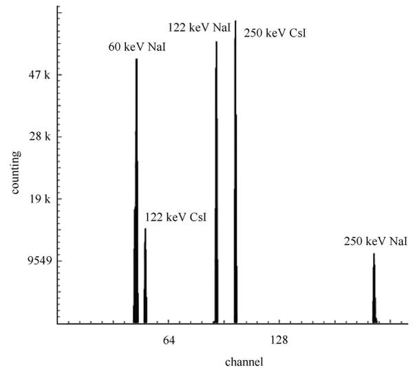
Fig. 8. The energy spectrum of the simulated NaI(Tl)/CsI(Na) detection of the 60 keV, 122 keV and 250 keV X-ray photoelectrons.
