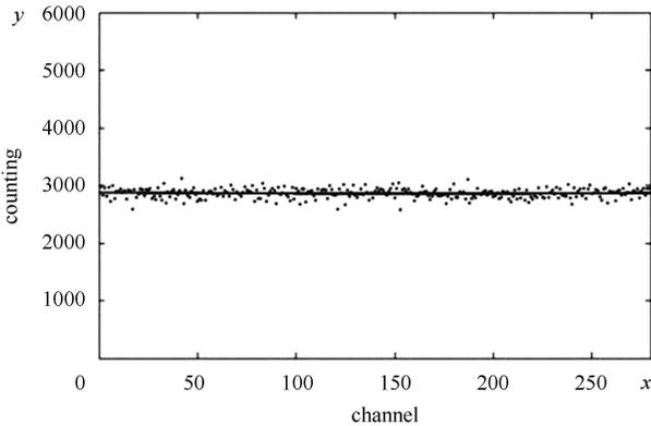
Fig. 6. Equiprobability random statistical distribution generated by the random number module. ( $\delta_i = y_i - \bar{y}$ , the standard deviation of  $\delta_i$  is 89.81, which is about 3% of the mean counting value  $\bar{y}$ ).
