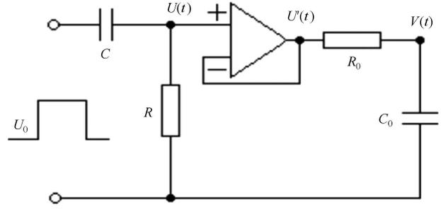
Fig. 4. The design drawing of detector signal simulation [2].
