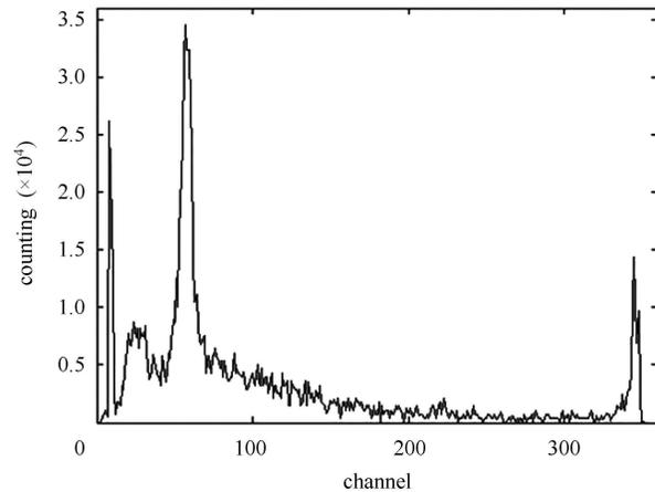
Fig. 10. The simulated energy spectrum of  $^{241}\text{Am}$  radioactive source in NaI and CsI scintillation crystals.
