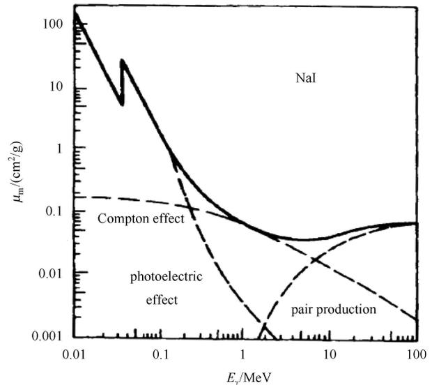
Fig. 1. The mass-absorption coefficient of NaI crystal [4].
