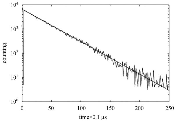
Fig. 11. The fitting chart of the signal time-interval (the fitting function  $f(x)=6533\exp(-0.03x)$ ,  $R$ -square=0.9983).
