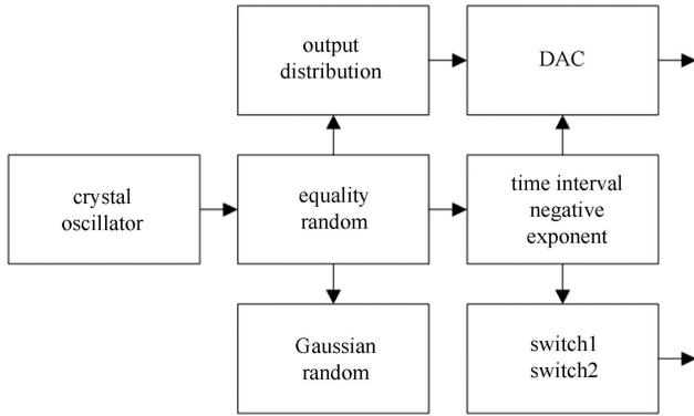
Fig. 3. Diagrammatic drawing of FPGA inside.
