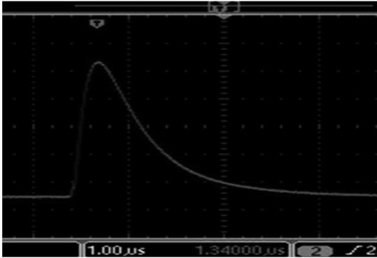
Fig. 5. The oscilloscope screenshot of the NaI wave.
