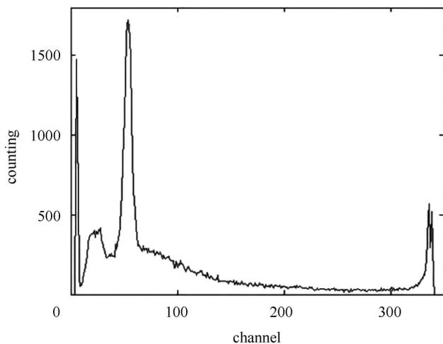
Fig. 9. The energy spectrum of  $^{241}\text{Am}$  radioactive source measured in NaI and CsI scintillation crystals.
