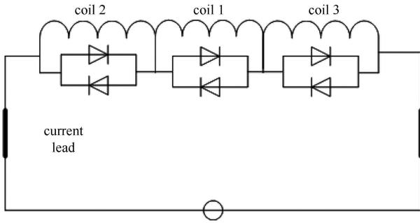
Fig. 9. Quench protection circuit.
