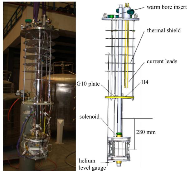
Fig. 8. (colour online) Assembly of test insert for CADs solenoid.
