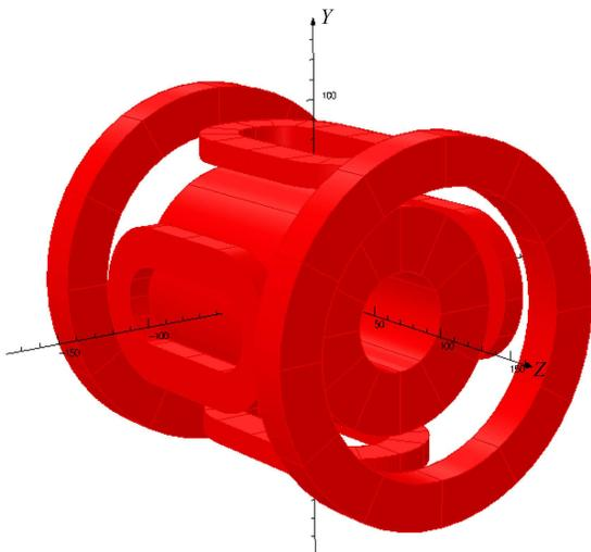
Fig. 5. (colour online) Coils configuration of the CADs solenoid.
