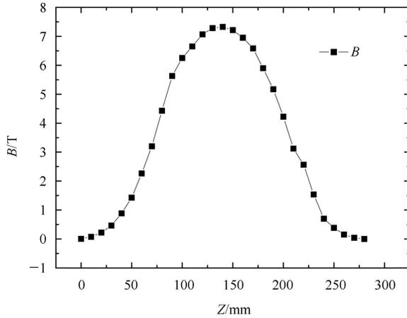
Fig. 10. The measured magnetic field distribution along the axis of the solenoid.
