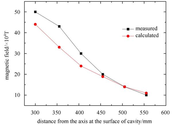
Fig. 11. Comparison between the measured fringe field and the calculated value.
