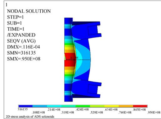
Fig. 7. (colour online) Simulated stress distribution of the solenoid caused by the electromagnetic forces.
