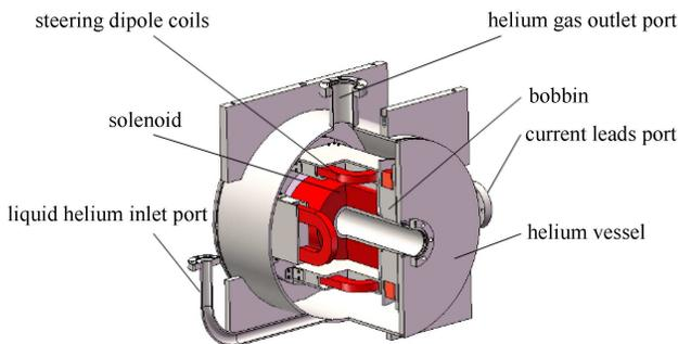
Fig. 6. (colour online) CADs solenoid assembly.
