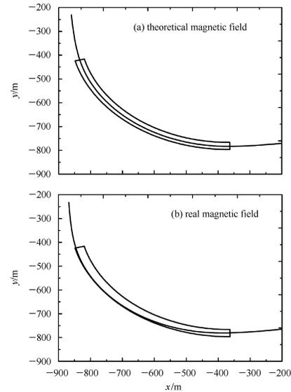
Fig. 2. Central particle orbit of MSi3 in the theoretical field and real isochronous magnet field.
