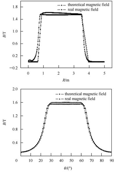
Fig. 1. R and  $\theta$  direction magnet distributions of measured and soft-edge approximations.
