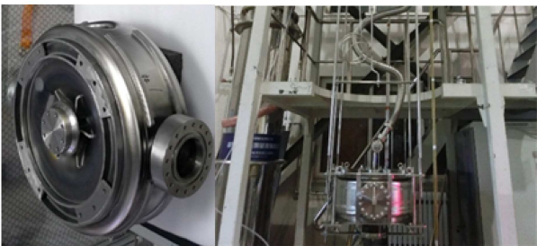
Fig. 7. Spoke012 cavity (left) and spoke012 cavity installed in vertical test stand (right).
