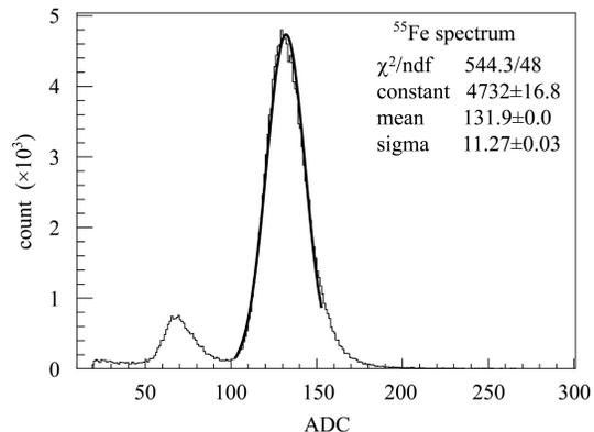
Fig. 3. A typical  $^{55}\text{Fe}$  energy spectrum, in Ar/isobutane(95/5) mixture. The energy resolution is  $2.35 \times 11.27 / 131.9 = 20.08\%$ .
