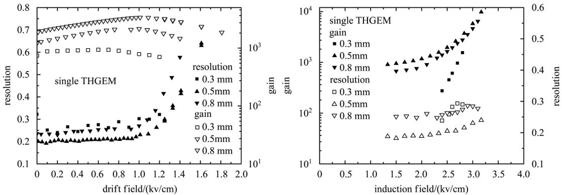
Fig. 4. The influences of drift (left) and induction (right) fields on the gain and resolution in an Ar/isobutane(95/5) mixture. The THGEM thickness is 0.5 mm and the voltage is 595 V.
