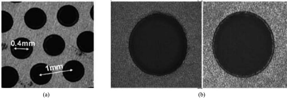
Fig. 1. Images of the THGEM plates. (a) The standard THGEM structure; (b) A single hole before (left) and after (right) the processes described in the text. The treated rim is less than 10  $\mu\text{m}$ .
