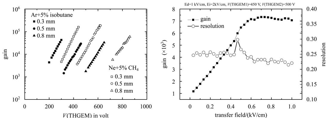
Fig. 5. The double-THGEM results. (left) The gain in different gases; (right) The influence of the transfer field. The gas is Ar/isobutane (95/5). The bad resolution at 0.45 kV/cm is due to some electromagnetic interference.
