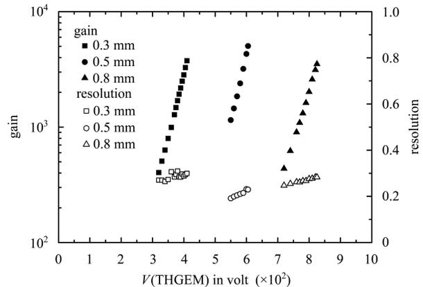
Fig. 2. The gain and energy resolution of single THGEM. In an Ar/isobutane(95/5) mixture, the drift field is 1 kV/cm and induction field 2.7 kV/cm.
