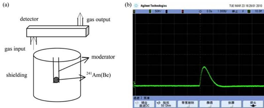
Fig. 6. The layout of the experimental setup and signal induced by thermal neutrons.
