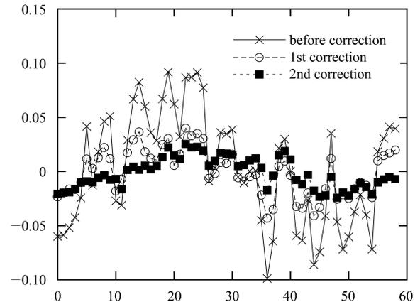
Fig. 2. Local coupling measurement and correction in the BER with the solenoid off. The horizontal axis is the BPM index and the vertical axis is the  $\bar{C}_{b,12}$ .
