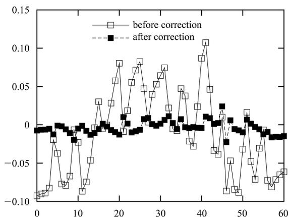
Fig. 3. Local coupling correction with the solenoid on. The horizontal axis is the BPM index and the vertical axis is the  $\bar{C}_{b,12}$ .
