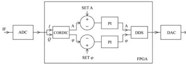
Fig. 3. Internal algorithm of the FPGA.
