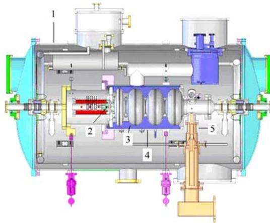
Fig. 1. The PKU SRF 3.5 cell photocathode injector. 1. Cryomodule, 2. Photocathode ( $\text{Cs}_2\text{Te}$ ), 3. 3.5 cell LG Nb cavity, 4. Liquid helium tank, 5. Main coupler.
