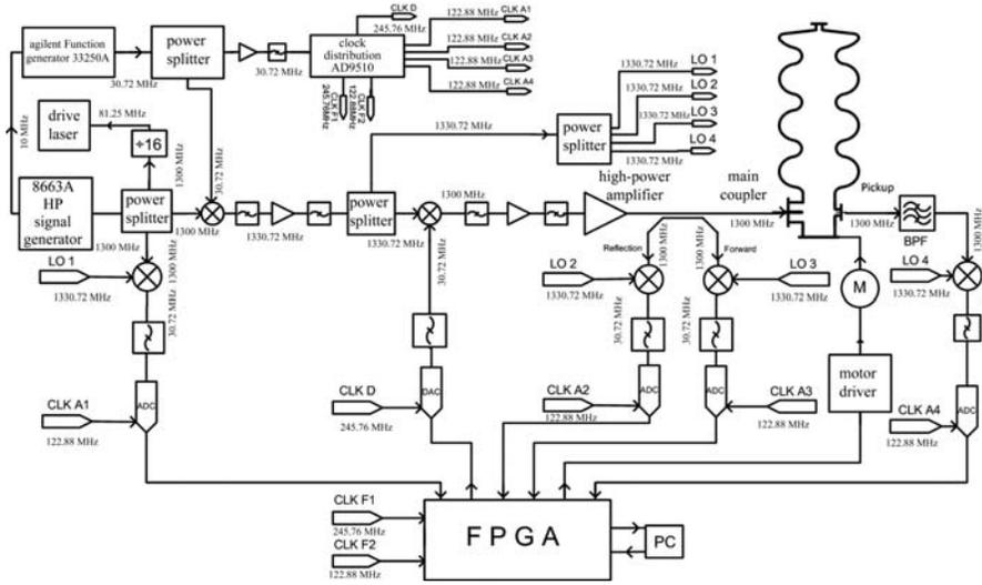
Fig. 2. The schematic of the control system for a PKU SRF photocathode injector.
