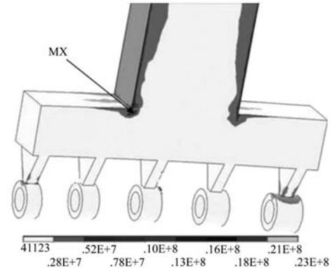
Fig. 6. Distribution of the thermal stress.
