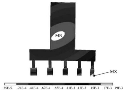
Fig. 5. Distribution of the displacement.
