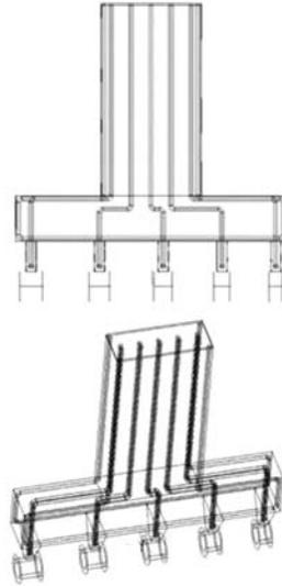
Fig. 3. The water cooling system (half model).
