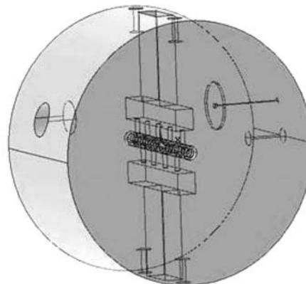
Fig. 1. The sketch drawing of DTL tank.
