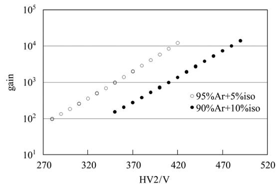
Fig. 3. The plot of detector gain with voltage.
