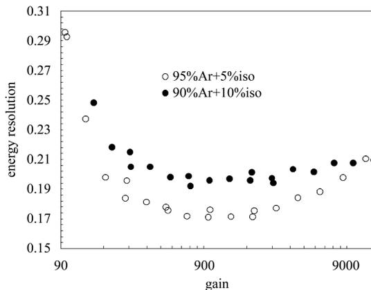
Fig. 5. The energy resolution changes with the gain.
