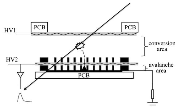
Fig. 1. A schematic diagram of the prototype detector.
