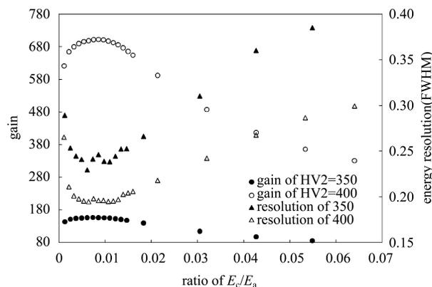
Fig. 6. The gain and energy resolution versus the ratio of  $E_c$  to  $E_a$ .
