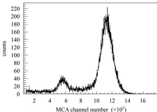
Fig. 4. The spectrum of  $^{55}\text{Fe}$  5.9 keV X-ray has an energy resolution of full energy peak which is 16% (FWHM). (95% argon, 5% isobutane).
