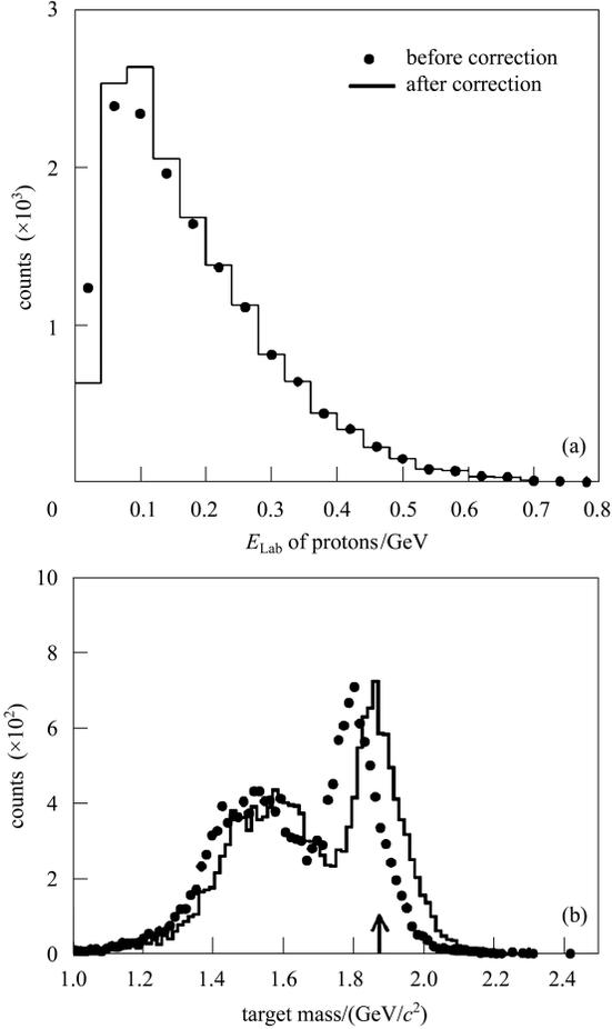
Fig. 2. Kinematical energy spectrum of protons (a) and reconstructed  $\gamma X \rightarrow \pi^- pp$  target mass (b) before and after correction for the material effect. In the right figure, there are two peaks, the wider and lower one was mainly contributed by multi-pion productions, and the narrower and higher one denotes the reaction of  $d(\gamma, \pi^- pp)$ ; the designed tagged photon energy was used for the target mass reconstruction, and the arrow indicates a deuteron mass.
