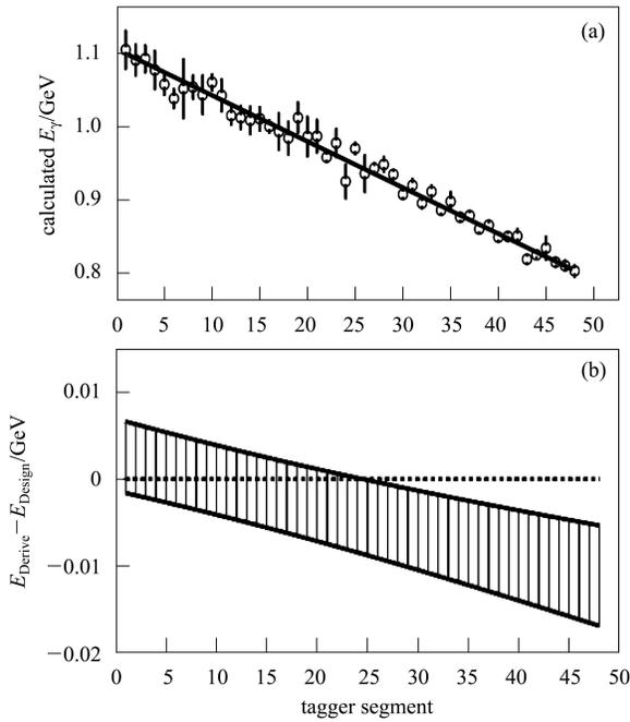
Fig. 5. Calibration of the photon tagging system. The errors showing in the (a) are the fitting error for each segment, the curve is a linear fitting; the (b) figure gives the propagation of the fitting for derived  $E_\gamma$  respecting to the designed  $E_\gamma$ .
