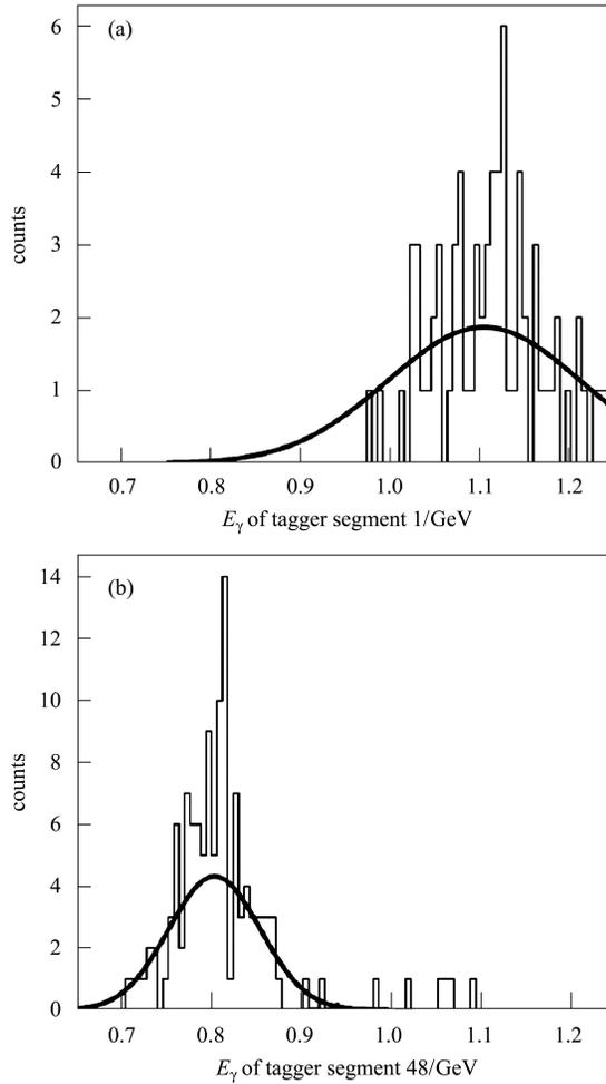
Fig. 4. The calculated  $E_\gamma$  for tagger segments 1 and 48. The curves are Gaussian fitting.
