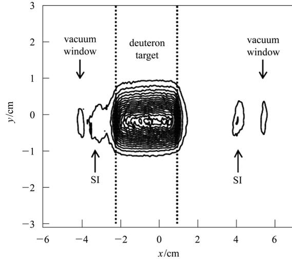
Fig. 3. Selection of vertex position. The  $x$  axis is along the photon beam line, and the  $y$  axis is vertical to the beam line, as described in Fig. 1. The broken lines indicate the selected target region. The SI (Super Insulation) and vacuum windows are also seen.
