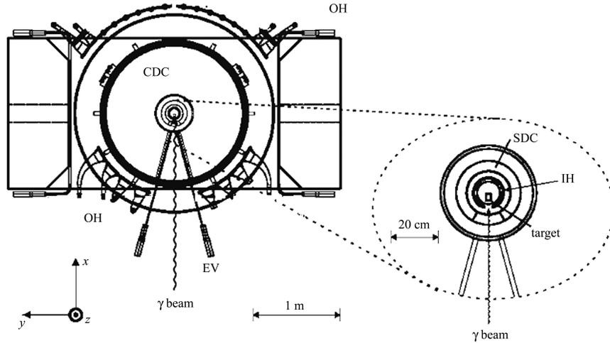
Fig. 1. Schematic drawing of NKS2. See details in the text.
