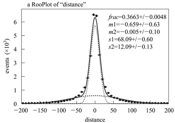
Fig. 4. Fitting of distance distribution with a double Gaussian function.
