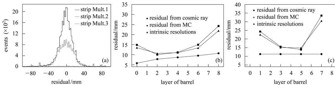
Fig. 3. Graph (a) is the residual distributions for different multiplicities for gap0 in the barrel. (b) and (c) are the residual distributions for the even and odd layers.
